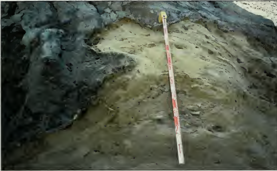
Figure 15 Folded basal contact of Tiskilwa sequence till (Oakland facies, Fig. 18) with underlying sand (Ashmore Tongue).
