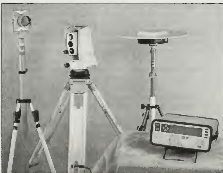
Figure D-2 Trimble 4000 GPS dual frequency receiver with "pizza dish" antenna and TTS 500 total station.
