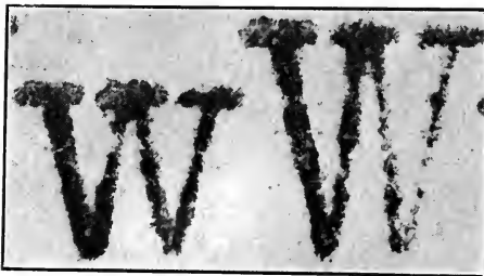
FIG. 185—Upper and lower case W's printing heavily on left.
