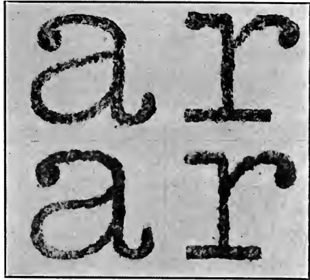
FIG. 179—Enlargement to show slight but distinctive divergence in design of Remington and Monarch letters.
