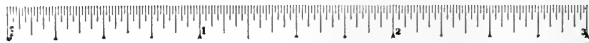
FIG. 20—Photographic Enlargement Measure, graduated in 64ths of an inch, to be photographed with the object to serve as a permanent record of the degree of enlargement.
