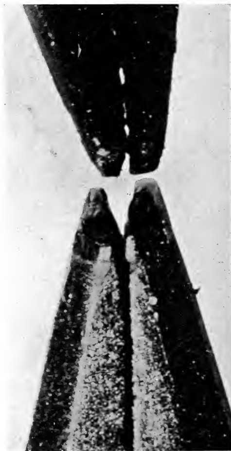
FIG. 78—Comparison of width of pen points. Gold pen with special point and old corroded steel pen. From exhibit in Matter of Frederick C. Hewitt will, Owego, N. Y. Photograph enlarged sixty diameters.
