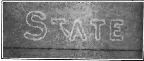
FIG. 153—Illustration of an accident to a watermark.
