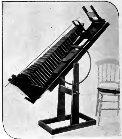
FIG. 14—Tilting Camera Stand in position for transmitted light photographs.
