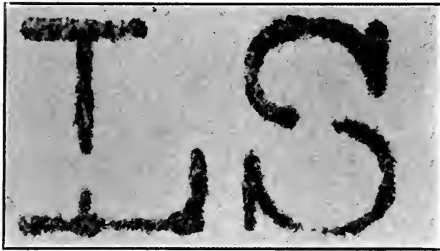
FIG. 188—Defective letters on a new machine.
