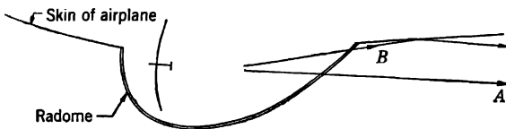
FIG. 9-15.—Reflection from the skin of an airplane.
