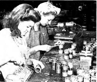
THIS BLIND MAN'S SKILLED FINGERS ARE CONTRIBUTING TO WAR PRODUCTION IN THE BCA VICTOR PLANT AT CAM-DEN, N. J. ASSEMBLY WORK ON TRANSMITTER COILS (BELOW) IS PERFORMED BY GIRLS IN THE NEW YORK PLANT OF RADIOMARINE CORPORATION OF AMERICA.
