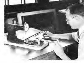
R. LEUSCHNER TESTS AN ASPHERICAL LENS (ABOVE) FOR DEVIATIONS FROM THEORETICAL DESIGN; THE AUTHOR REMOVES A PLASTIC ASPHERICAL LENS (BELOW) FROM THE MOLD IN WHICH IT WAS MADE.
