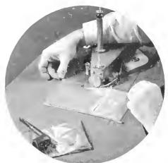
A TOBACCO POUCH MADE OF THERMO-PLASTIC MATERIAL IS "STITCHED" TO-GETHER IN A DEMONSTRATION OF RCA'S ELECTRONIC SEWING MACHINE.
