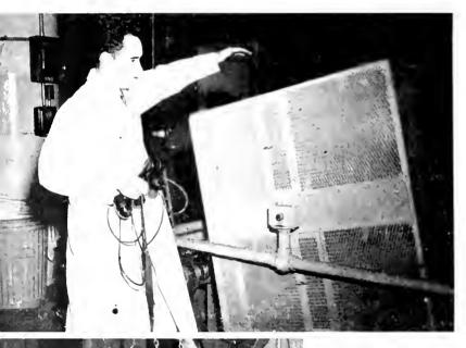
equipment is placed. A revolving hose directs a stream of water around the equipment. The nozzle is regulated so that the water may be made to fall in a gentle sprinkle or at a 55-mile per hour blast, duplicating the breaking of waves against the ship while a storm is raging. Some form of this test, according to York, is given to nearly all equipment to be exposed to the elements.
