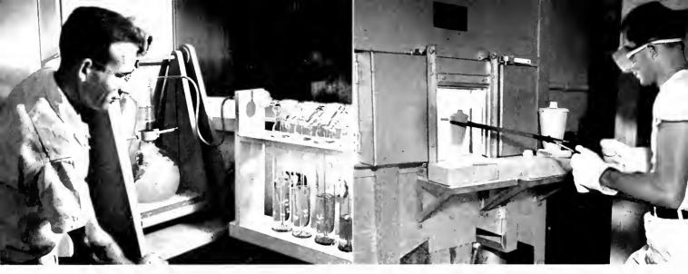
E. J. WOOD, RESEARCH CHEMIST, MANIPULATES A BUBBLING GAS TO PURIFY A SOLUTION WHICH IS BEING ELECTRICALLY HEATED AND SHAKEN IN THE PYREX FLASK.
