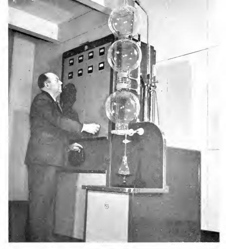
DR. GEORGE II. BROWN GIVES THE PENICILLIN ELECTRONIC DEHYDRATING APPARATUS HE DEVELOPED IN RCA LABORATORIES A FINAL INSPECTION BEFORE IT IS SHIPPED TO THE E. R. SQUIBE & SONS PLANT AT NEW BRUNSWICK, N. J.
