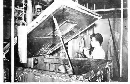
SALT SPRAY AND ULTRA-VIOLET RAYS PLAY ON NAVY COMMUNICATIONS EQUIPMENT IN THIS TEST (ABOVE) TO DETERMINE ITS CORROSION RESISTANCE. EQUIPMENT IS CHECKED FOR WATER-TIGHTNESS AFTER IT HAS BEEN SUBMERGED IN A LARGE TANK (BELOW) FOR A NUMBER OF HOURS.
