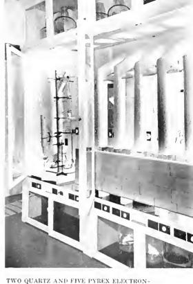
TWO QUARTZ AND FIVE PYREX ELECTRON-ICALLY-CONTROLLED STILLS FURNISH QUADRUPLY DISTILLED WATER AND ACIDS—THE "LIFEBLOOD" OF LABORATORY OPERATIONS.
