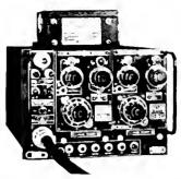
RCA Aviation Radio Transmitter used in the PBY Catalino
