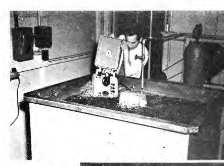
BECAUSE NAVY TELEPHONES MUST NOT FAIL AT CRUCIAL MOMENTS, THEY ARE TESTED (RIGHT) UNDER SIMULATED STORM CONDITIONS, IN THIS SCENE (BELOW), SHIPPOARD COMMUNICATIONS EQUIPMENT IS UNDERGOING A 55-MILE-AN-HOUR BLAST FROM A WATER HOSE IN A SUA-WATER SPLASH TEST.
