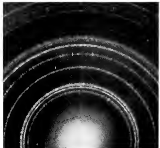
PATTERN OF ZINC OXIDE SMOKE PARTICLES SHOWS RING CONSTRUCTION.
