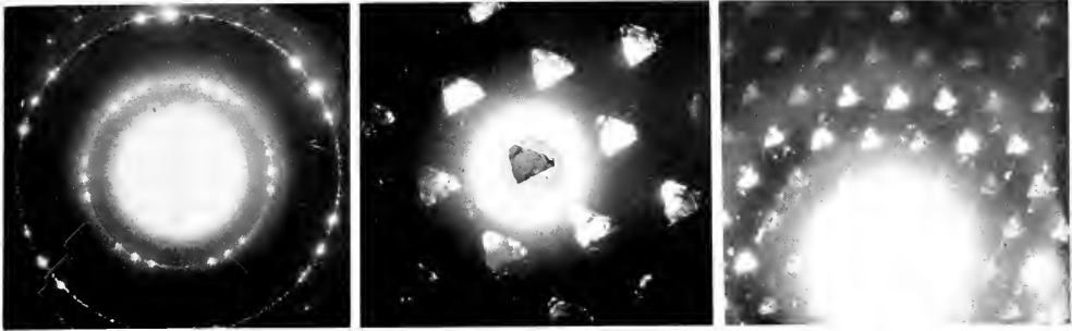
LEFT: CRYSTALS OF GRAPHITE AS THEY APPEAR UNDER THE DIFFRACTION CAMERA. THE SYMMETRY OF THE BEADS IS A RESULT OF THE HEXAGONAL STRUCTURE OF GRAPHITE. CENTER: COMBINATION ELECTRON MICROSCOPE AND ELECTRON DIFFRACTION PATTERN OF A SINGLE FLAKE OF GRAPHITE. THE CENTER IS A TRUE ELECTRON MICROGRAPH AT ABOUT 5,000 MAGNIFICATION. RIGHT: DIFFRACTION PATTERN OF BAUXITE CRYSTALS.
