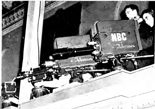
RCA IMAGE ORTHICON CAMERAS INSTALLED IN GALLERY OF THE HOUSE OF REPRESENTATIVES ARE TRAINED ON THE SPEAKER'S STAND.
