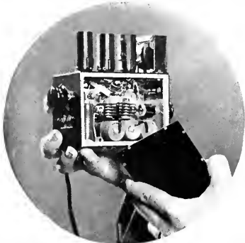
DEVELOPMENT MODEL OF INEXPENSIVE RADIO FREQUENCY CONVERTER WHICH ENABLES BLACK-AND-WHITE TELEVISION RECEIVERS TO REPRODUCE COLOR PROGRAMS IN MONOCHROME.
