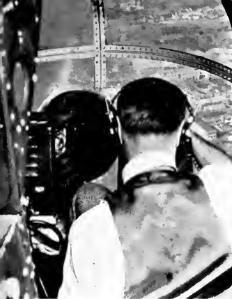
TELEVISION CAMERA OPERATOR POINTS THE SENSITIVE ICONOSCOPE THROUGH NOSE OF PLANE TO PICK UP TERRAIN BENEATH. RIGHT: DIAGRAM SHOWING HOW AIRBORNE TELEVISION SYSTEM WOULD BE UTILIZED IN AN AMPHIBIOUS OPERATION TO TRANSMIT SCENE OF ACTION TO COMMAND POSTS ON SHIP OR LAND.
