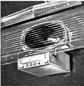
USE OF SMALL TUBES HAS GREATLY REDUCED THE DIMENSIONS OF AUTOMOBILE RADIOS AND IMPROVED THEIR PERFORMANCE IN BOTH PRIVATE CARS AND COMMERCIAL VEHICLES.
