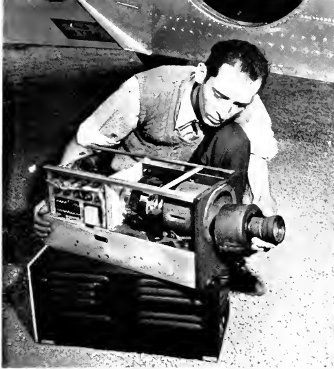
BY SKILLFUL DESIGN, ELEMENTS OF THE "BLOCK" SYSTEM HAVE BEEN COMPRESSED INTO THE 50-POUND UNIT SHOWN ABOVE AT LEFT. RIGHT: THE SAME EQUIPMENT INSTALLED IN ITS PLACE IN THE PLANE'S NOSE.
