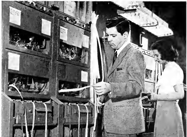
TAPES PASSING THROUGH THIS "PACKAGE SET" AT THE CENTRAL RADIO OFFICE MAY CARRY RADIOTELEGRAPH MESSAGES ARRIVING IN NEW YORK FROM MOSCOW OR ON THEIR WAY TO THE RUSSIAN CAPITAL.
