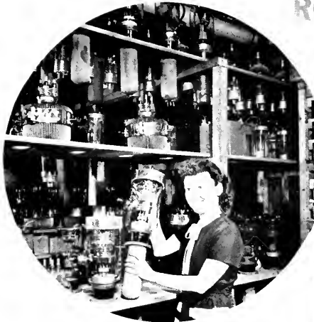
LARGE WATER-COOLED ELECTRON TUBES EMPOWER THE "VOICE" OF THE POWERFUL TRANSMITTERS AT ROCKY POINT.
