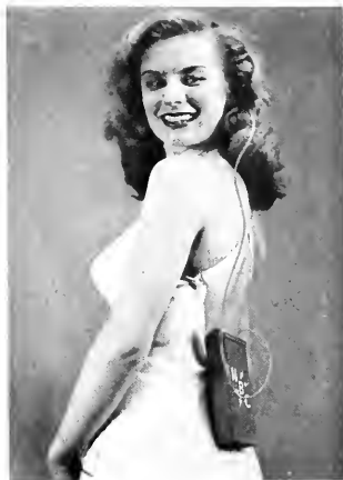
THE WIRE LEADING FROM COMPACT RECEIVER TO EAR IS ALSO THE ANTENNA WHICH PICKS UP THE SIGNALS FROM A TRANSMITTER IN THE STUDIO CEILING.
