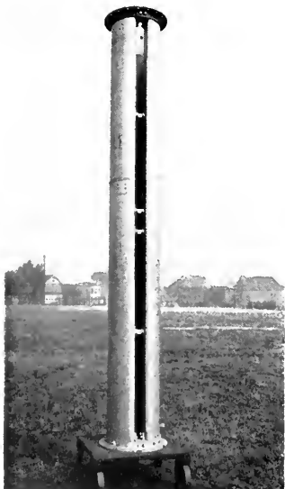
THE NEW PYLON ANTENNA, A ROLLED-STEEL CYLINDER WITH A LONGITUDINAL SLOT, DELIVERS A HIGHER POWER GAIN THAN ANY OTHER TYPE OF FM ANTENNA.
