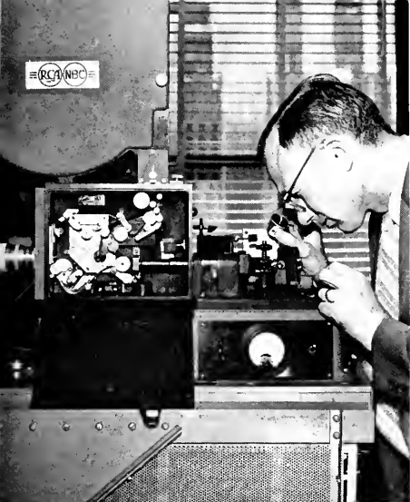
RALPH LOVELL EXAMINES THE MECHANISM WHICH APPLIES THE SOUND RECORDING TO THE EDGE OF THE FILM CONTAINING THE TELEVISION RECORDING.
