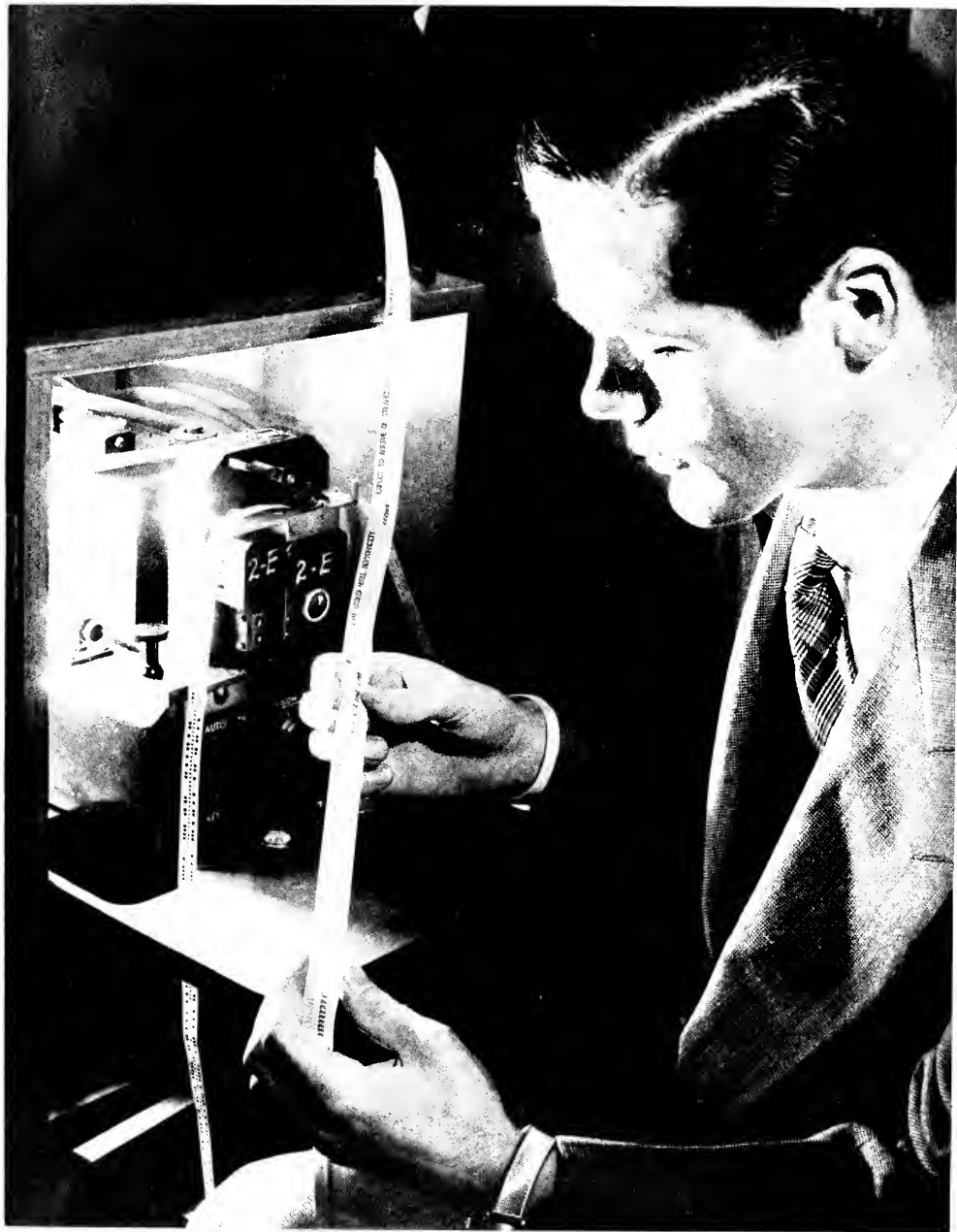
RADIOTELEGRAPH MESSAGES IN MORSE CODE ON TAPE ARE AUTOMATICALLY TRANSLATED INTO TELETYPE CODE BY THIS MACHINE AT RCA COMMUNICATIONS, INC.
