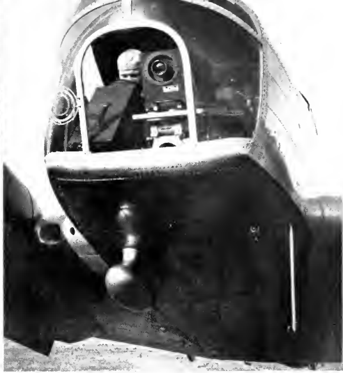
BY SKILLFUL DESIGN, ELEMENTS OF THE "BLOCK" SYSTEM HAVE BEEN COMPRESSED INTO THE 50-POUND UNIT SHOWN ABOVE AT LEFT. RIGHT: THE SAME EQUIPMENT INSTALLED IN ITS PLACE IN THE PLANE'S NOSE.
