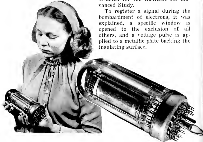
SMALL SIZE OF THE "SELECTRON" TUBE BELIES ITS UNUSUAL POWERS OF "MEMORY" IN HELPING TO SOLVE COMPLEX MATHEMATICAL PROBLEMS.
