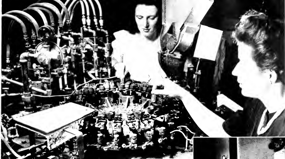
THIS MACHINE SEALS A PIECE OF GLASS TUBING TO THE TOP OF EACH MINIATURE TUBE SO THAT AIR AND GASSES INSIDE THE ENVELOPE MAY BE EXHAUSTED.
