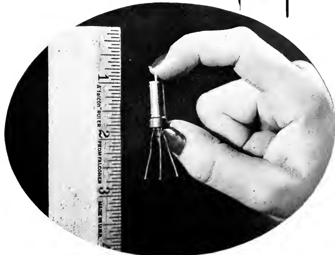
BELOW: THIS VIEW SHOWS THE COMPACT SIZE OF THE VIBROTRON. PROTRUDING THROUGH THE TOP OF THE TUBE IS THE ROD OR LEVER WHICH TRANSFERS MECHANICAL MOTION FROM THE OUTSIDE INTO THE HIGH VACUUM OF THE INNER CHAMBER, AS PICTURED IN THE SKETCH AT THE RIGHT
