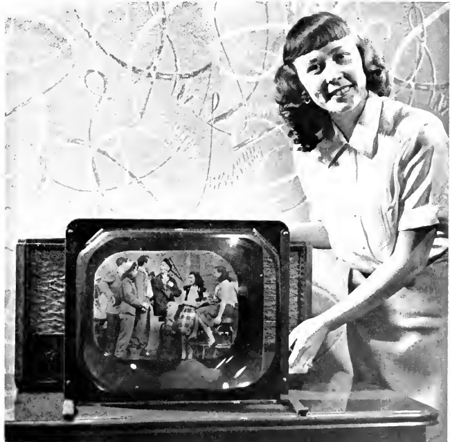
TELEVISION IMAGE MAGNIFIER IN PLACE IN FRONT OF THE SCREEN OF AN RCA VICTOR MODEL STS30.
