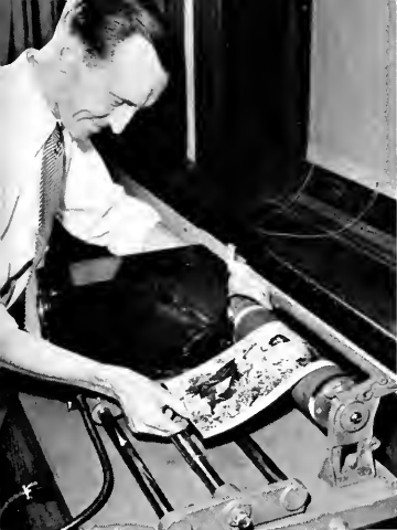
PRINCIPAL ELEMENTS OF THE MODERN RADIOPHOTO SYSTEM ARE THE ROTATING CYLINDER, THE LEAD SCREW (CENTER ROD OF THE THREE) AND THE SCANNING OR RECORDING HEAD IN THE BLACK BOX.
