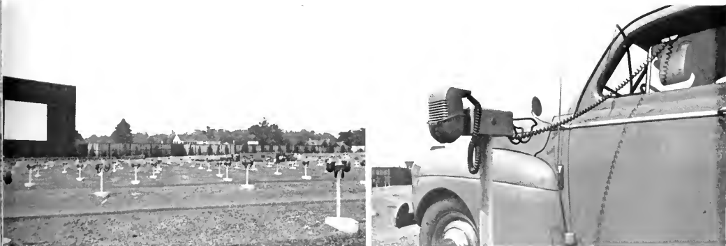
LOUD SPEAKERS WHICH CAN BE DRAWN THROUGH CAR WINDOWS ARE SHOWN BELOW ON THEIR PARKING-LOT PEDESTALS. AT RIGHT: AN IN-CAR SPEAKER HAS BEEN LIFTED OFF ITS PEDESTAL AND HOOKED ONTO THE INSIDE OF A CAR WINDOW
