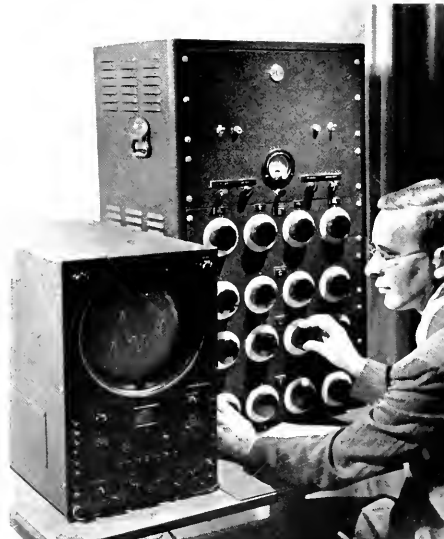
PROBLEMS OF LOCATING AND ARRANGING ANTENNAS CAN BE SOLVED IN A FEW MINUTES BY THIS ELECTRONIC DEVICE.
