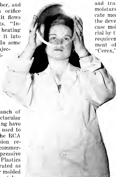
A PLASTIC TELEVISION PROJECTION LENS IS CHECKED FOR FLAWS.
