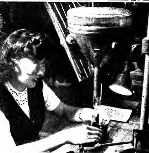
BELOW: NON-REFLECTING CARBON COATING IS APPLIED TO INTERIOR OF TUBE BY LONG-HANDLED BRUSH TO KEEP STRAY ELECTRONS FROM THE PICTURE SCREEN.
