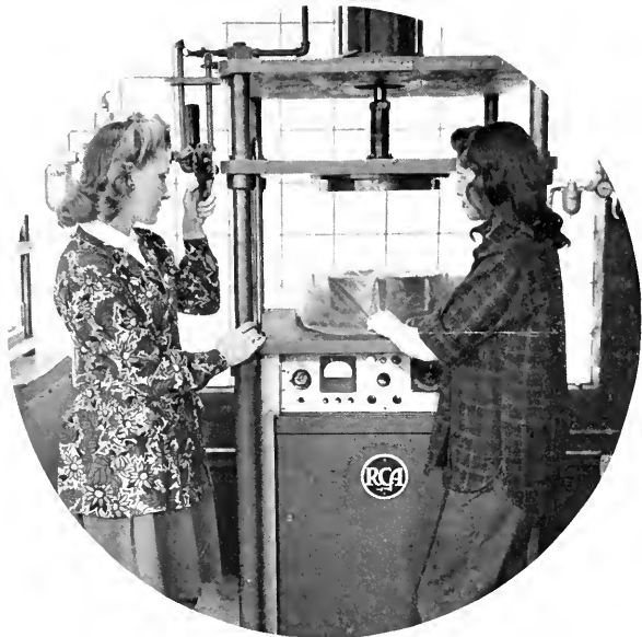
OPERATORS AT THE DU PAGE PLANT, LOMBARD, ILL., JOIN VINYLITE STRIPS BY ELECTRONIC HEAT-SEALING TO FORM AN AIRTIGHT, WATERTIGHT BALLOON.
