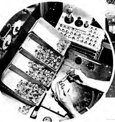
A HIGH DEGREE OF SKILL IS NEEDED TO ASSEMBLE THE SMALL ACORN TYPE TUBES (LEFT) AND ELEMENTS OF THE LARGER TUBES (ABOVE).
