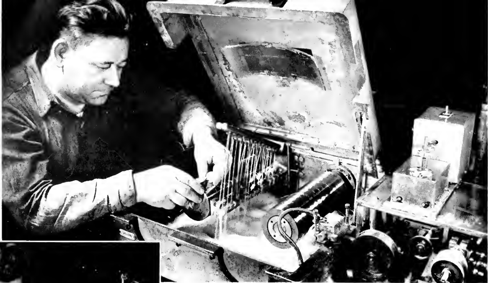
FILAMENTS FOR MINIATURE TUBES ARE MADE BY RUNNING WIRE AS FINE AS SILK THROUGH THE DIAMOND DIES OF THIS MACHINE WHICH REDUCES THE WIRE DIAMETER TO ONE THIRD THE THICKNESS OF HUMAN HAIR.
