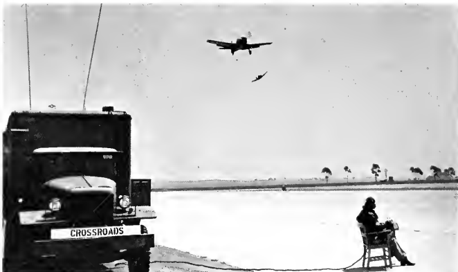
TOWERS SIMILAR TO THE ONE ABOVE SUPPORTED TELEVISION CAMERAS AND TRANSMITTERS ON BIKINI. AT RIGHT: "DRONE" PLANE CARRYING A TELEVISION CAMERA, COMES IN FOR A LANDING. OPERATOR IN FOREGROUND HAS TAKEN OVER CONTROL FROM THE "MOTHER" PLANE IN THE DISTANCE.
