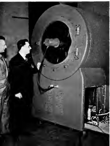
THE AUTHOR AND BARTON KREUZER, MANAGER OF RCA THEATRE AND RECORDING EQUIPMENT, EXAMINE A TELEVISION PROJECTOR GIVING A 15 BY 20-FOOT SCREEN IMAGE.
