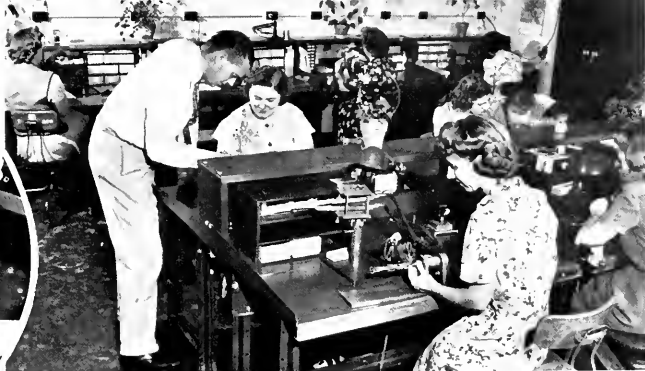
A HIGH DEGREE OF SKILL IS NEEDED TO ASSEMBLE THE SMALL ACORN TYPE TUBES (LEFT) AND ELEMENTS OF THE LARGER TUBES (ABOVE).
