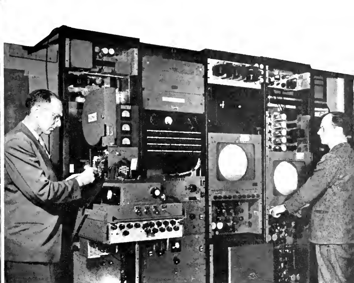
COMPLETE TELEVISION RECORDING EQUIPMENT INCLUDING CAMERA AT EXTREME LEFT WITH SOUND RECORDING AND MONITORING PANELS.
