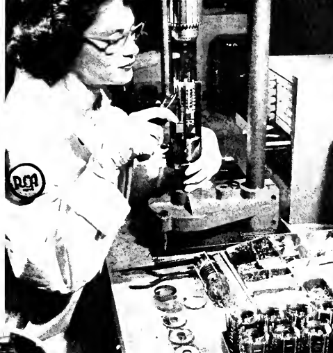
CATHODE RAY "GUN" IS ADDED TO THE IMAGE ORTHICON CAMERA TUBE.
