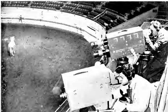
NBC ANNOUNCER BEN GRAUER AND USHERETTE BETTY BEUHLER DEMONSTRATE HIGH SENSITIVITY OF IMAGE ORTHICON USING ILLUMINATION OF ONE CANDLE. BELOW: GREATLY SUPERIOR SENSITIVITY OF CAMERA USING THE IMAGE ORTHICON (BACKGROUND) IS COMPARED WITH PERFORMANCE OF CONVENTIONAL CAMERA IN PICKING UP SCENES FROM THE RODEO AT MADISON SQUARE GARDEN.
