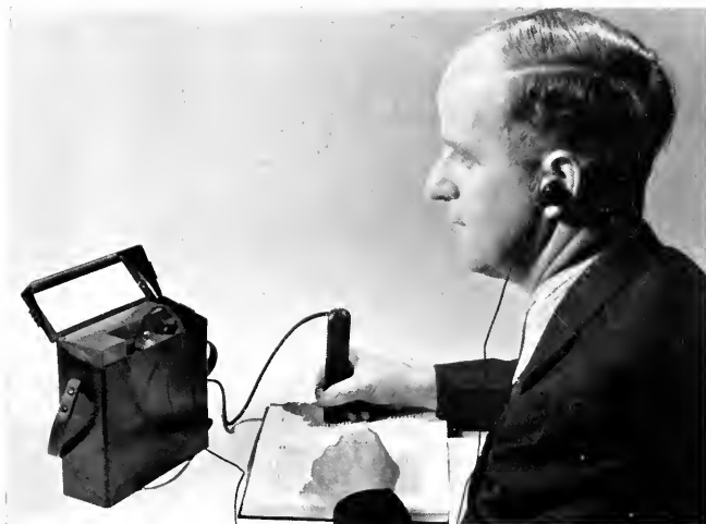
A HAND-HELD STYLUS, MOVED ACROSS A LINE OF PRINTED TYPE, CONVERTS LETTERS AND WORDS INTO RECOGNIZABLE SOUNDS BY ELECTRONIC ACTION.
