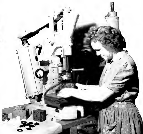
ONE OF THE POWERFUL PRESSES AT THE RCA VICTOR PLANT TURNING OUT PLASTIC PARTS FOR RADIOS.
