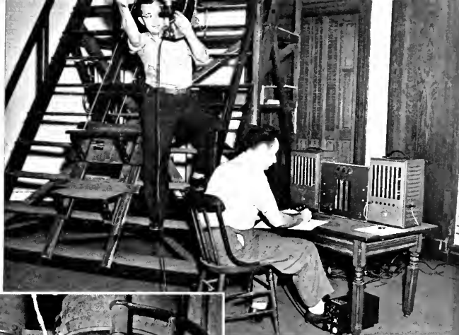
ABOVE: WITH AN ACCURACY OF ONE MILLIONTH SECOND, RCA ELECTRONIC INTERVAL COUNTERS ON TABLE MEASURE ELECTRON PULSES GENERATED BY THE FAINTEST STARLIGHT.
