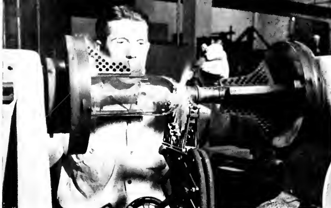
HEAT IS APPLIED TO JUNCTION OF GLASS AND METAL AS ONE STEP IN MAKING A VACUUM-TIGHT SEAL. BELOW: A COMPLETED SEAL BETWEEN TWO METAL TERMINALS AND A GLASS SUPPORT.
