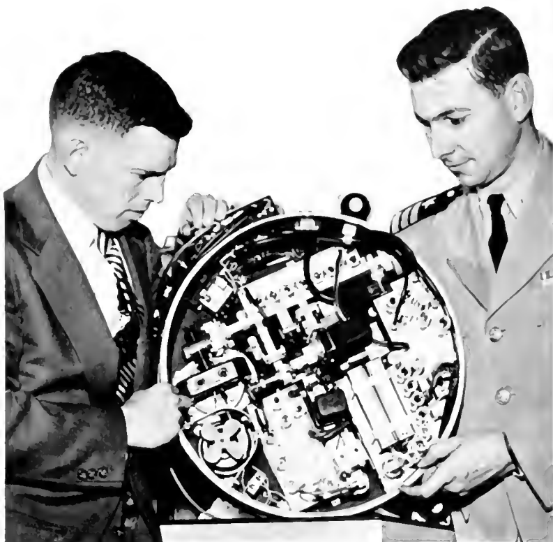
W. B. Kirkpatrick, manager of RCA Victor's Government Radar Unit, and Commander M. A. Mason, head of the Navy Bureau of Aeronautics Radar Section, examine transmitter-receiver unit of new radar.
