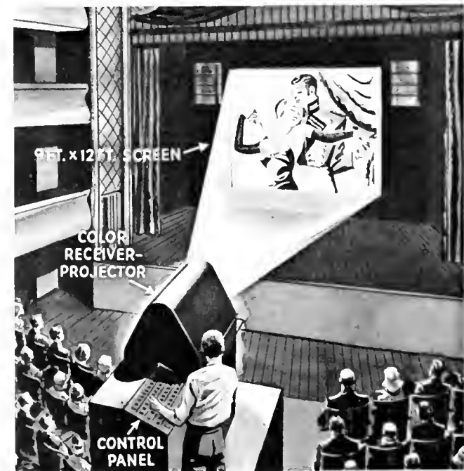
Artist's interpretation of the large-screen color television apparatus installed in the Colonial Theatre, New York, for the October field tests.
