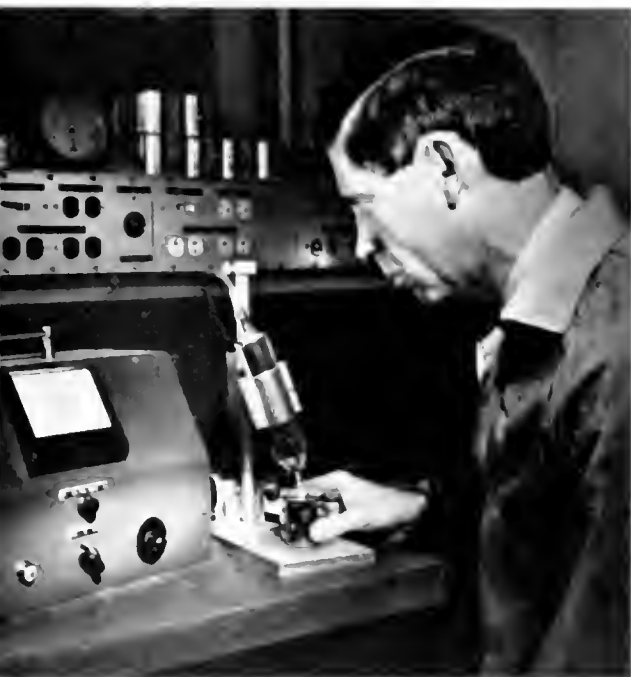
Dr. J. G. Woodward of RCA Laboratories Division demonstrates vibrating plate viscometer.
