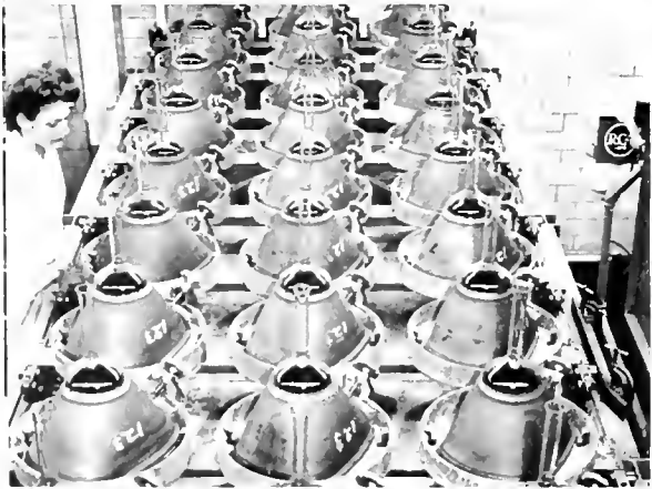
Tubes move slowly on this travelling belt while the fluorescent powder becomes a flawless surface on the glass face-plate.
