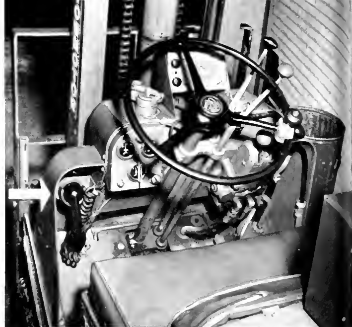
Headsets for the fork lifts are placed at the left of the operator with the transmitter-receiver installed behind the seat (extreme right).
