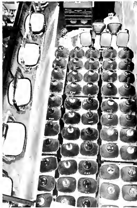
An elevated conveyor transports the 17-inch rectangular tubes from one process to another.
