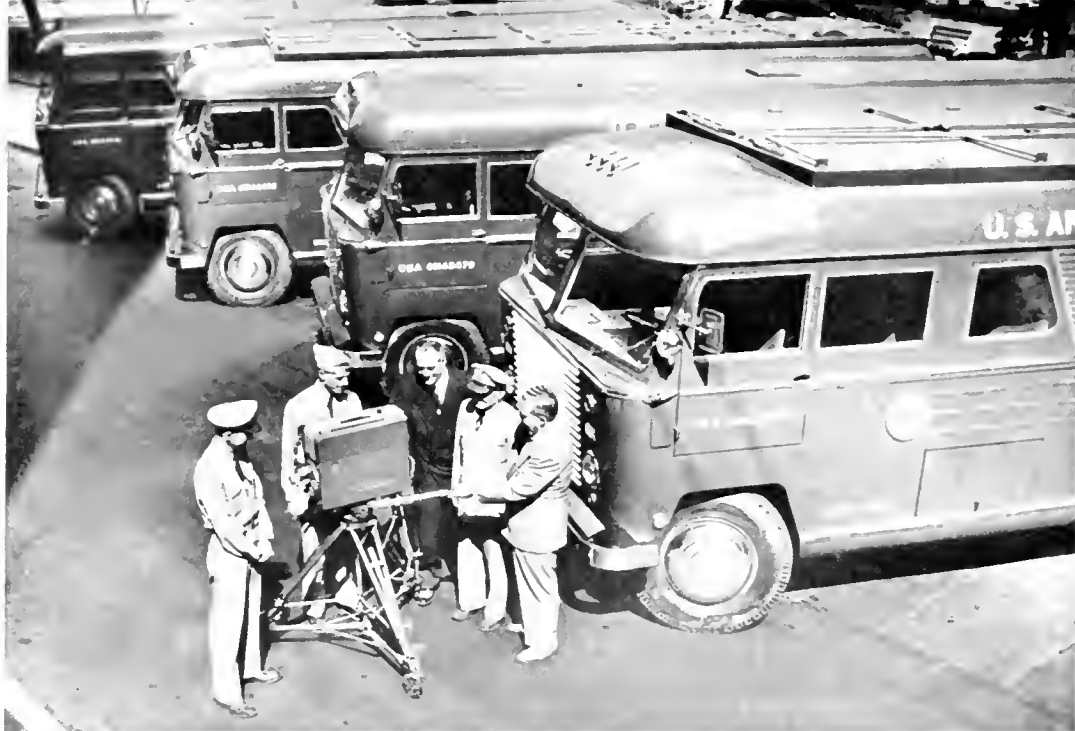
Four huge vans comprise the modern "TV station on wheels" developed by RCA for the U. S. Army Signal Corps.
