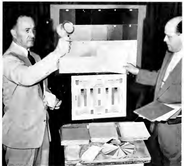
The author (left) measures the temperature of the studio illumination as Cliff Stiegelbauer holds a red-orange card against a gray scale. The comparison shows that this particular hue will be reproduced on TV screens as Munsell \approx 7 gray.
