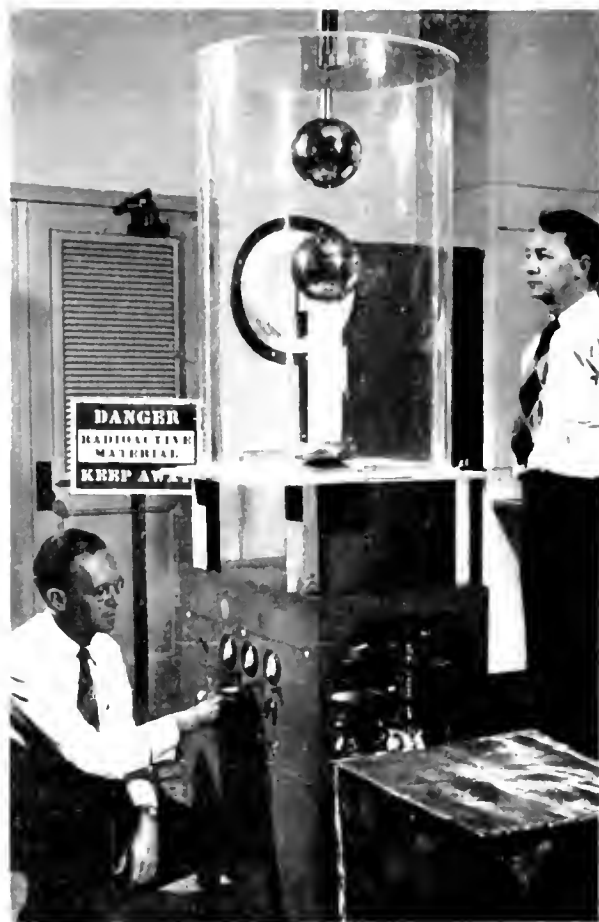
RCA SCIENTISTS EXPERIMENT WITH A HIGH-VOLTAGE GENERATOR, USING RADIOACTIVITY AS ITS SOURCE OF ENERGY.
