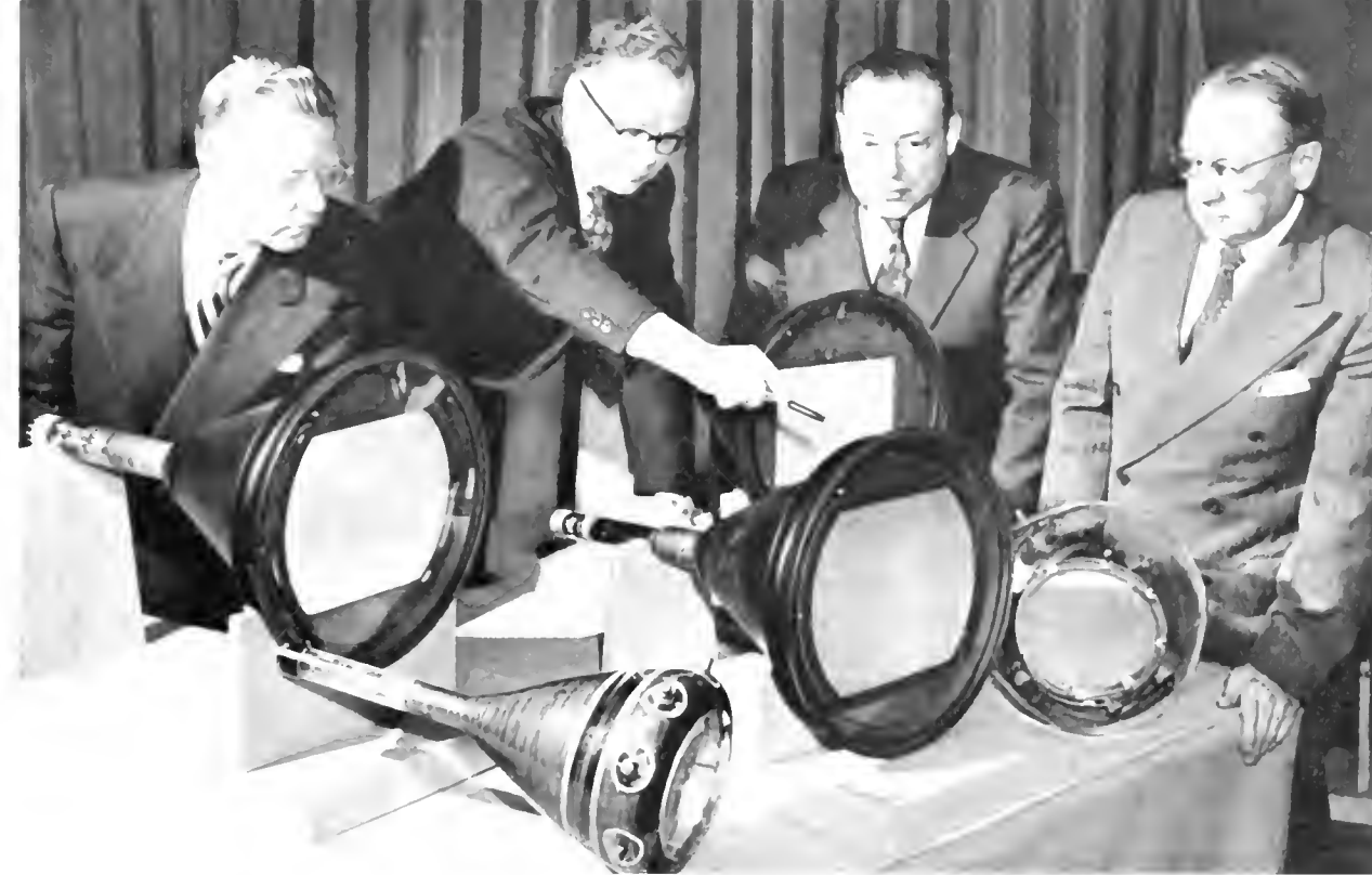
Four scientists of RCA examine five of the tri-color television picture tubes developed at the company's laboratories at Princeton, N.J., and Lancaster, Pa. They are: (left to right) E. W. Herold; Dr. E. W. Engstrom, Vice President in Charge of RCA Laboratories Division; H. B. Law, and Dr. V. K. Zworykin, Vice President and Technical Consultant of the Division.
