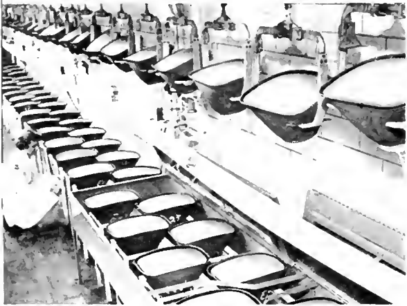
Fluorescent screen surfaces of television picture tubes are quick-dried in the special racks shown in foreground.
