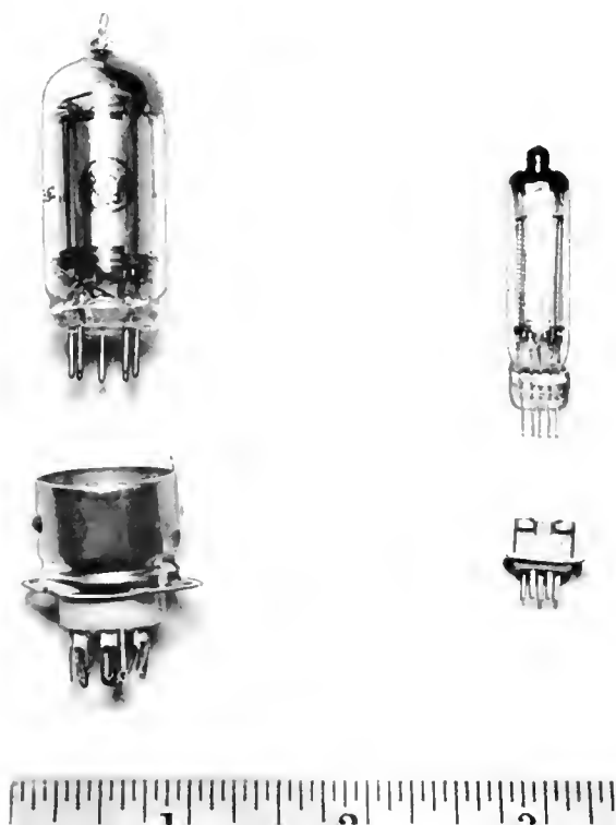
Tube-socket combinations from old (left) and new walkie-talkies emphasize the rapid progress in miniaturization of radio components.
