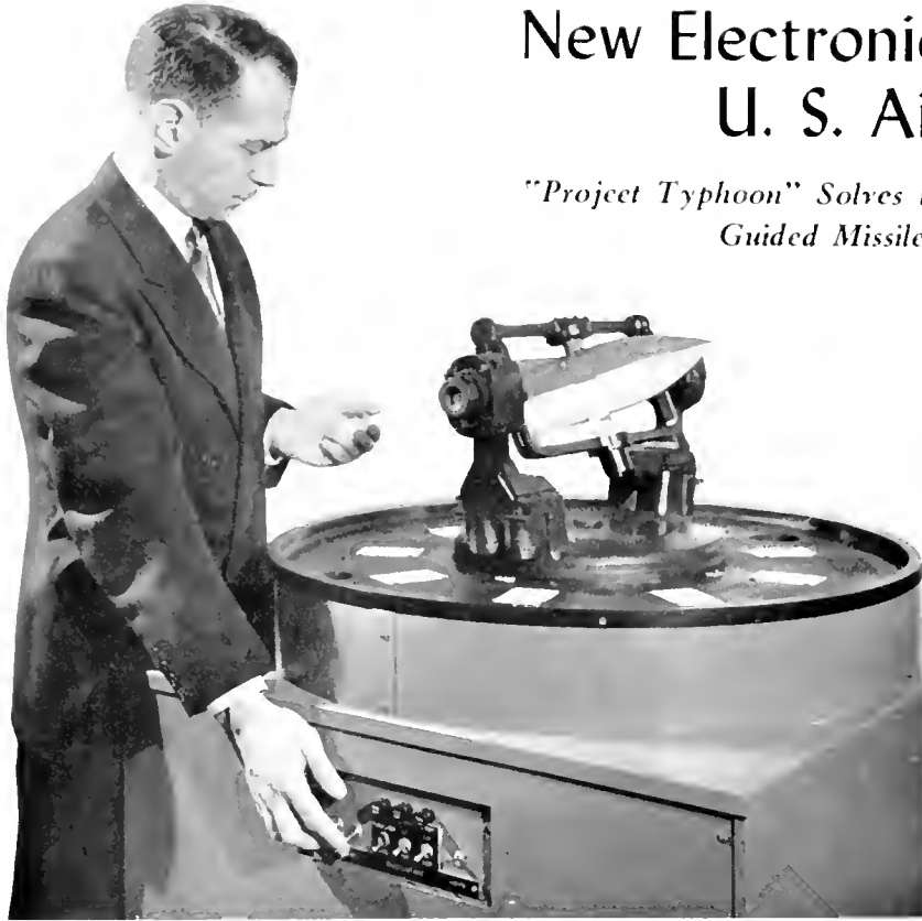
A PHYSICIST AT RCA LABORATORIES TIMES THE ACTION OF A MODEL USED TO SIMULATE THE BEHAVIOUR OF A GUIDED MISSILE UNDER FLIGHT CONDITIONS AS DETERMINED BY THE ANALOGUE COMPUTER DEVELOPED AT THE LABORATORIES.
