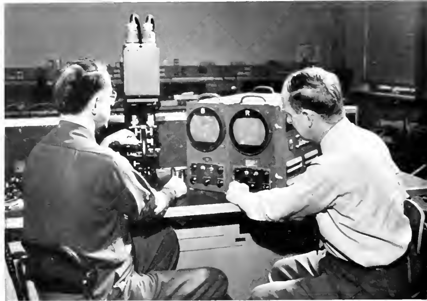
DR. A. K. PARPART (LEFT) AND L. E. FLORY DEMONSTRATE THE TELEVISION-MICROSCOPE COMBINATION WHICH PERMITS DIRECT OBSERVATION OF LIVING CELLS.
