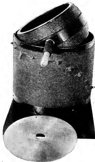
A SUITABLE VARIOCOUPLER For broadcasting or amateur reception, with its metal shield which reduces body capacity effects
