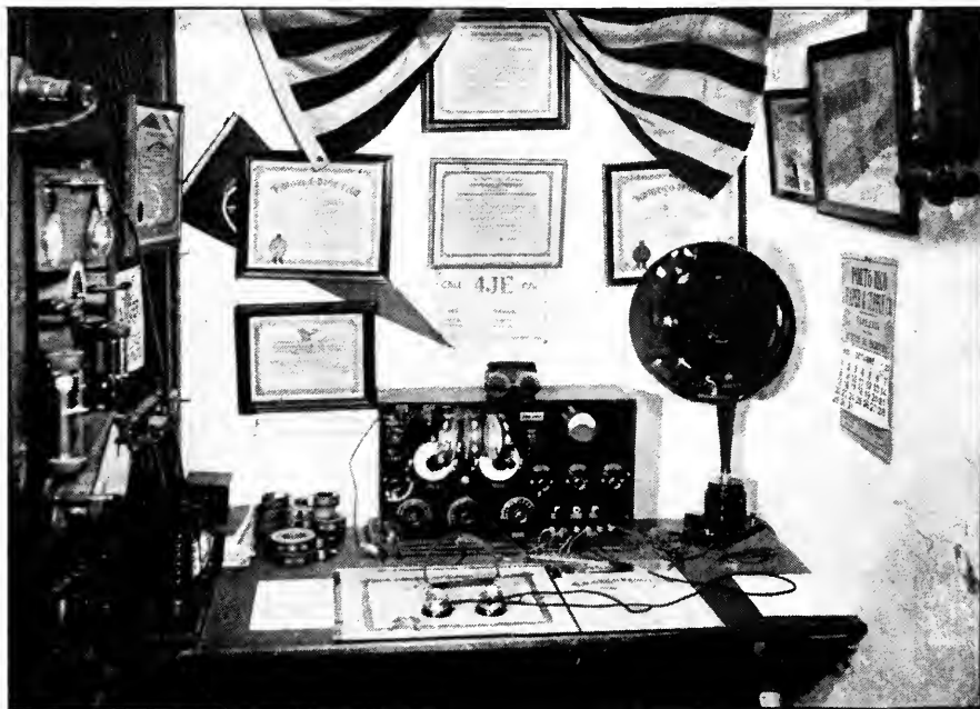
A PRE-WAR MULTI-RANGE RECEIVER Designed for transatlantic work with a single tube
