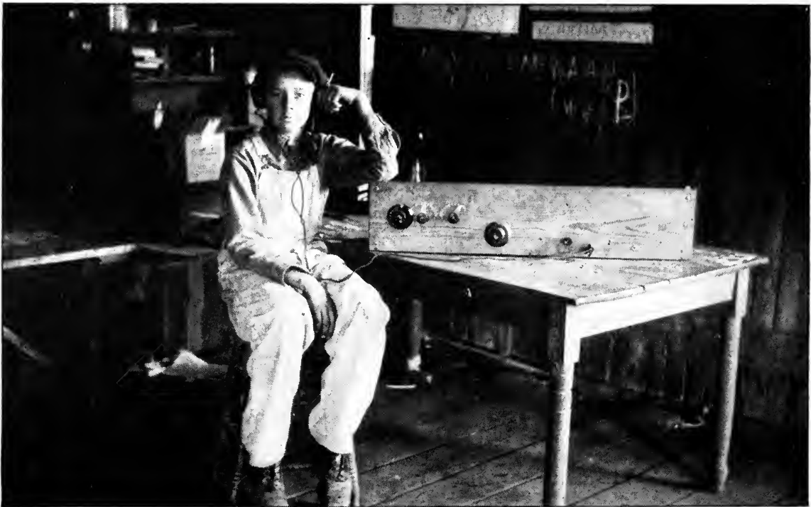
BILLIE ORR, OF YOAKUM, TEXAS, REACHES OUT MORE THAN 1000 MILES WITH THIS SET He saved up for a few simple parts, wound his inductance on a salt-box, salvaged some old telegraph wire for an aerial, used his dad's auto storage battery as the "A Batt.," and pulled in Detroit, Denver, and Atlanta. He has left plenty of room for the stage or so of amplification which he hopes to add
