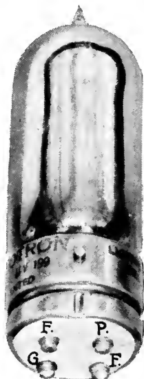
FIG. 3 Showing arrangement of contacts on the UV-199
