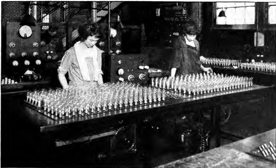
WD-11's and WD-12's on the aging table. The tubes are kept on this table one hour to increase the possible electron emission and to test for the degree of vacuum
