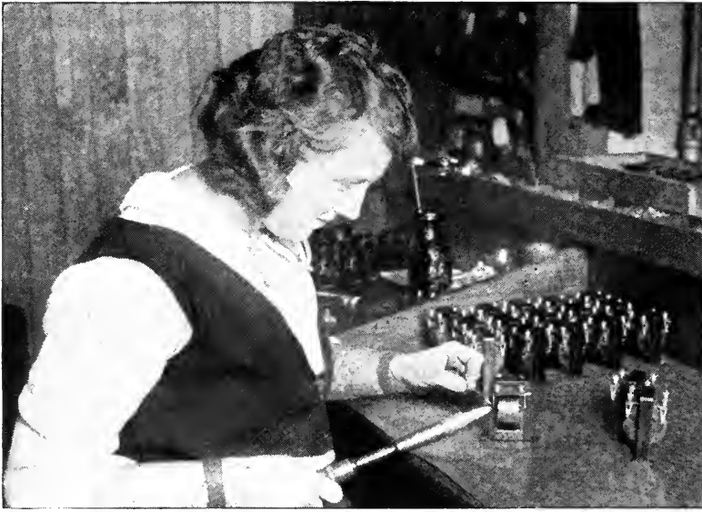
SOLDERING TRANSFORMER LEADS—A DELICATE JOB
