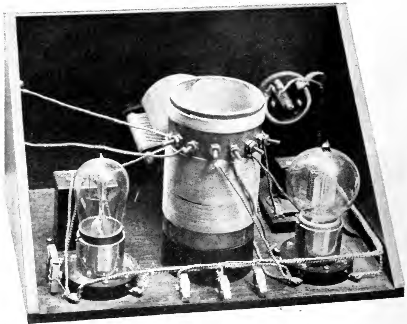
FIG. 7 Experimental type of wavemeter oscillator. The large coil is used as an oscillator, the smaller coil is a modulator creating an audible note. This type is not as convenient to construct as that shown in Figs. 5 and 6. This oscillator is made for use on a measuring bridge. It covers a wavelength band of 200 to 600 meters
