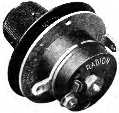
A NEUTRALIZING CONDENSER Which may be used in place of the two penny-size pieces of copper suggested for the neutralizing capacity for the first tube
