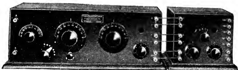
A THREE-CIRCUIT RECEIVER AND TWO-STEP AMPLIFIER With an outdoor antenna, it will operate a loud speaker over considerable distances
