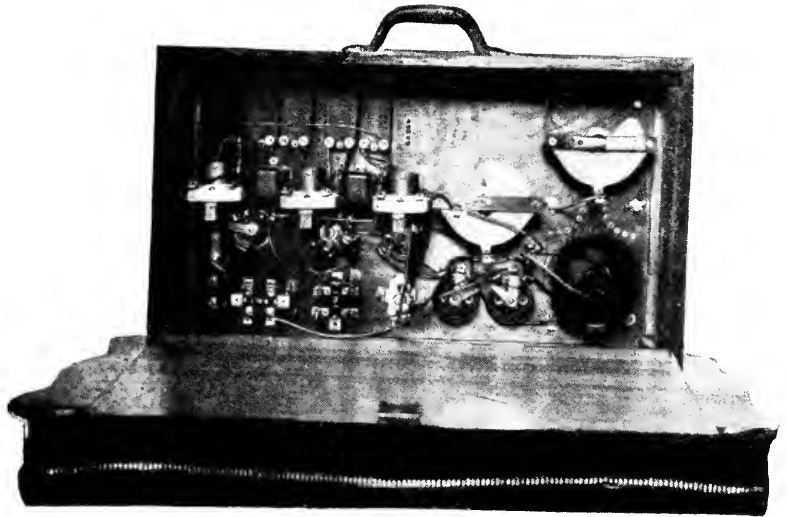
FIG. 4 The interior of the three-tube set. Plenty of room here, and no crowding of parts
