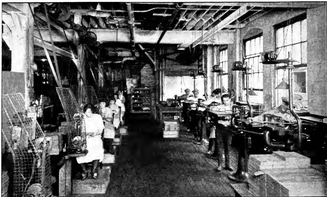
ENGRAVING AND FINISHING PANELS FOR FOUR-TUBE RECEIVERS
