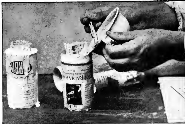
FIG. 5 Molding the porous cup
