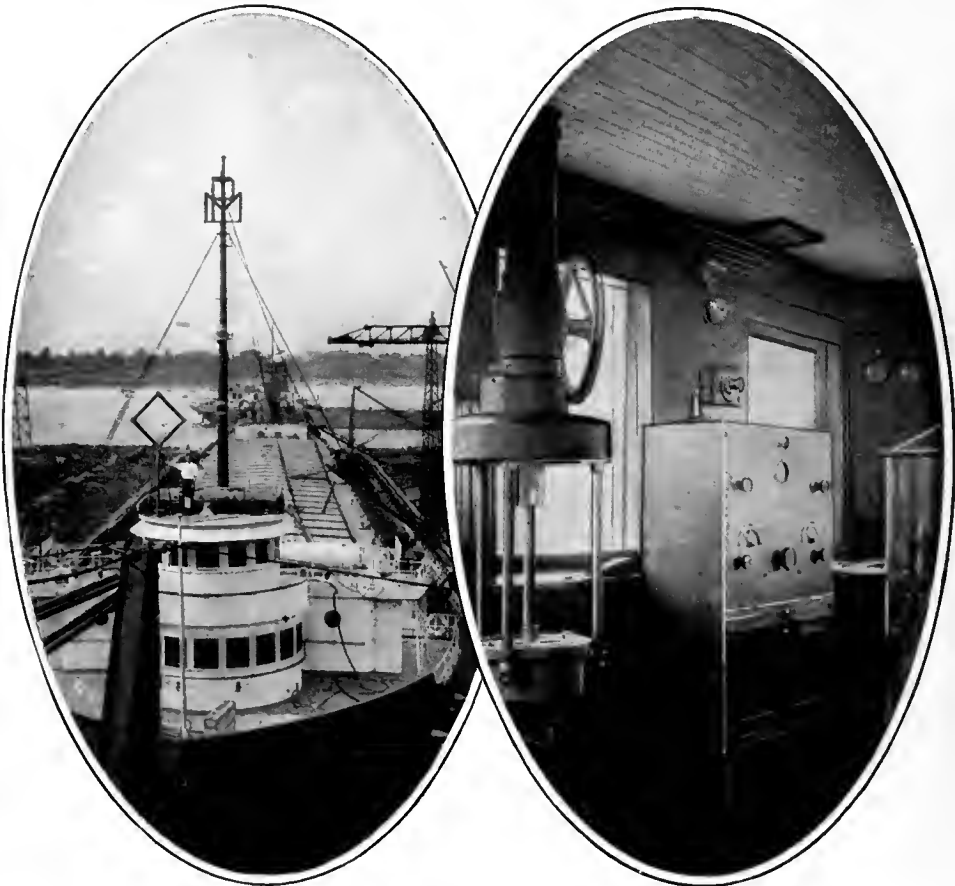
A RADIO COMPASS INSTALLATION ON A GREAT LAKES SHIP
