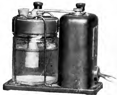
FIG. 4 The Balkite trickle charger enables any one to use his present A battery as a power unit. The photograph shows Balkite B Supply, trickle charger and Brach power control switch. The insert view shows the inside of the trickle charger and the chemical rectifier
