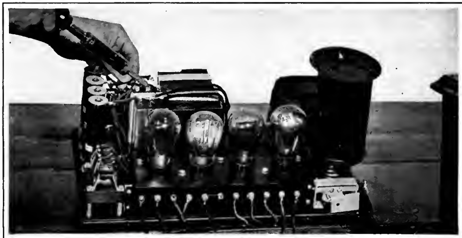
MAKING TESTS ON AN A. C. UNIT
