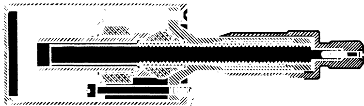
FIG. 55. Micrometer condenser (Ward and Pratt). There are three clamping bolts, only one of which is shown.
