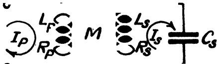
FIG. 15. Primary circuit and tuned secondary circuit.
