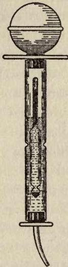
FIG. 62. The hydrometer syringe for determining electrical condition of the storage battery.
