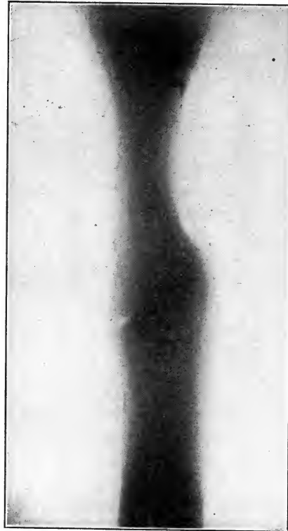
Radium picture. Tube of 15 grain of Radium 40 activity suspended one week above bone which was placed on a bare photographic plate.
