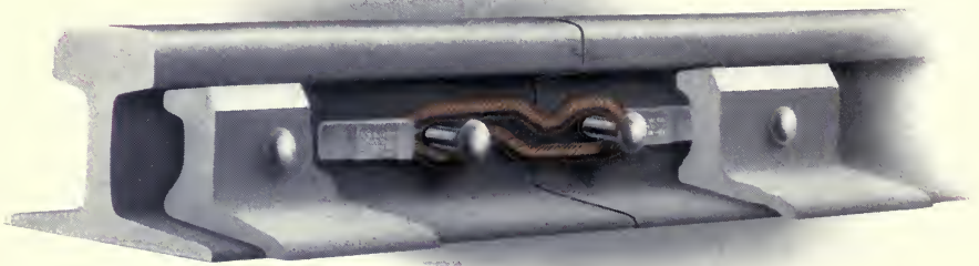
Showing a Soldered Bond Applied to Web of Rail
