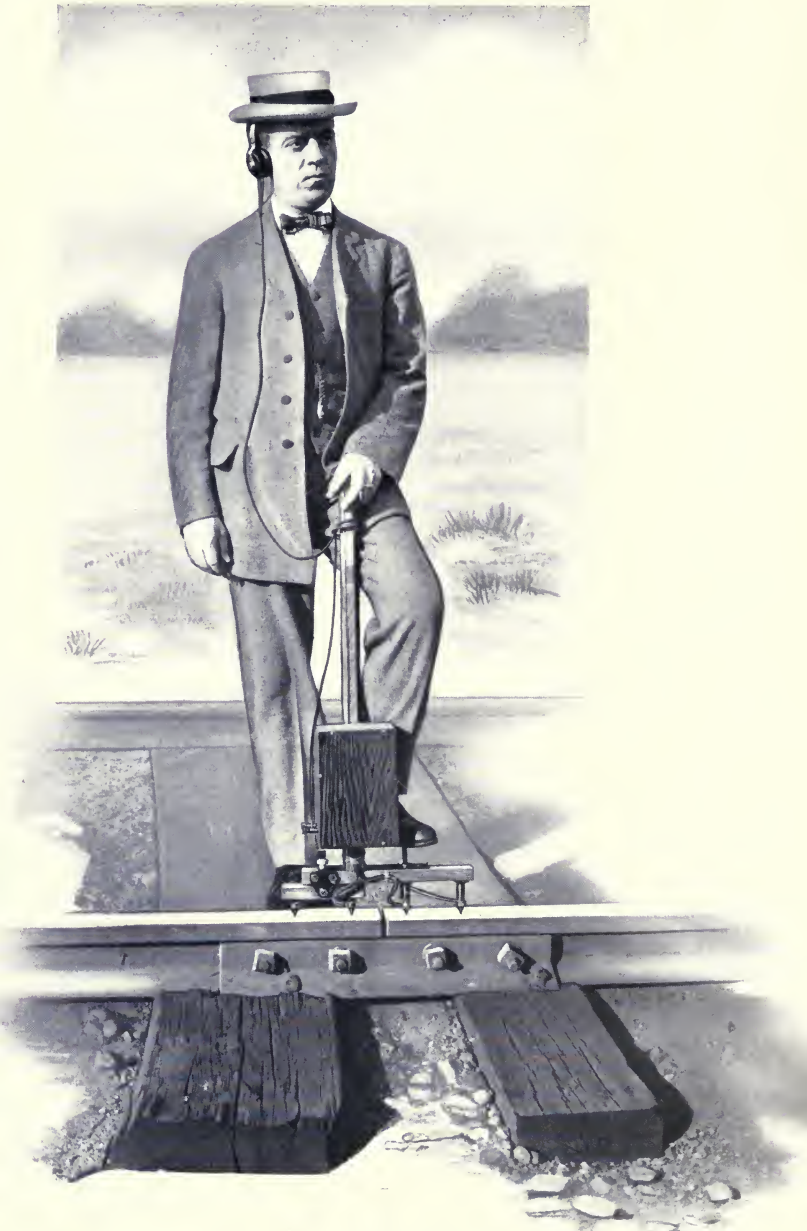
Operating a Crown Bond Tester
