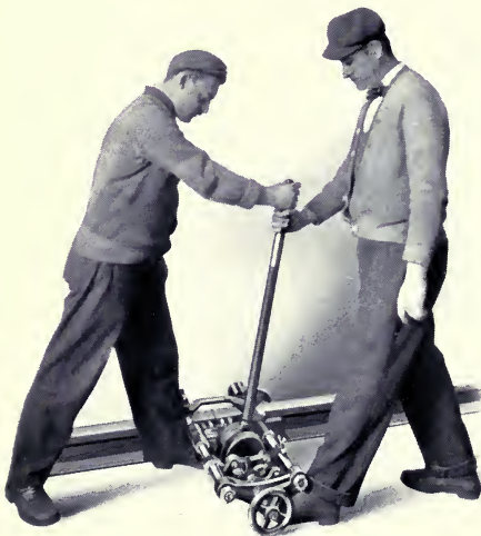
No. 22 Drill Being Operated by Two Men
