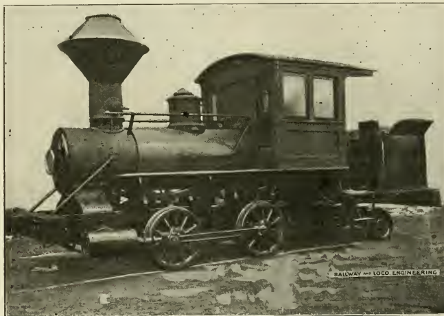
ENGINE WITH OSCILLATING CYLINDER AND NO VALVE GEAR
