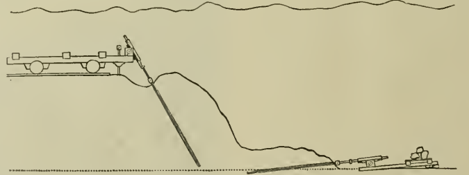
TAKING OUT BOTTOM BY HOLES DRILLED FROM HEADING AND ALONG FLOOR. (Reproduced from "Drinker's Tunneling.")
