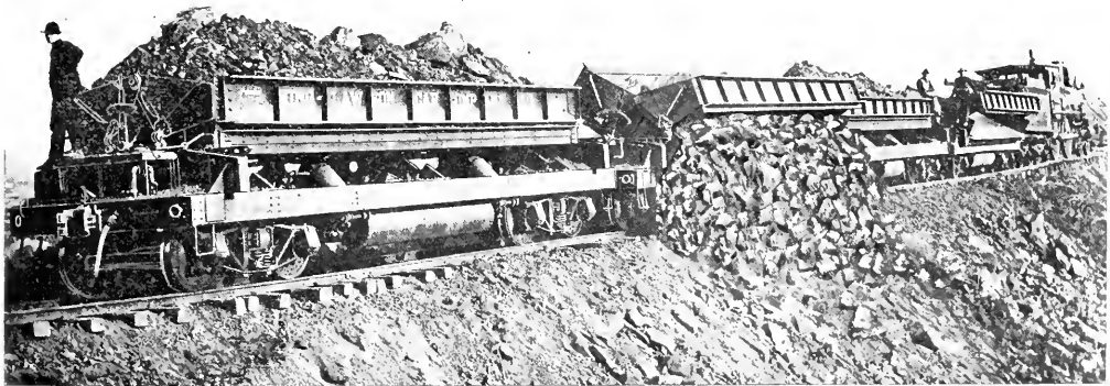
"CAUGHT WITH THE GOODS." INSTANTANEOUS PHOTOGRAPH OF THE KING-LAWSON CAR IN ACTION.
