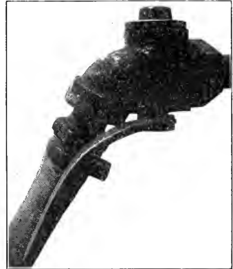
ANGLE VALVE—HOSE PROTECTING HANDLE.
