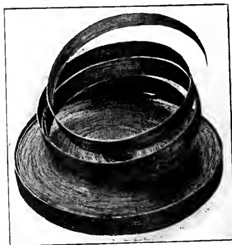
CHIP FROM CROSSHEAD PIN.
