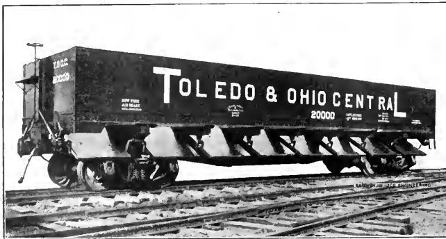
SIDE DUMP CAR, WITH ALL DROP DOORS FULL OPEN.
