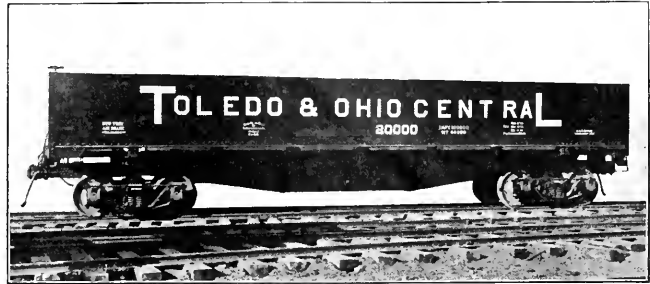
RALSTON DUMP CAR AS A GENERAL SERVICE GONDOLA.
