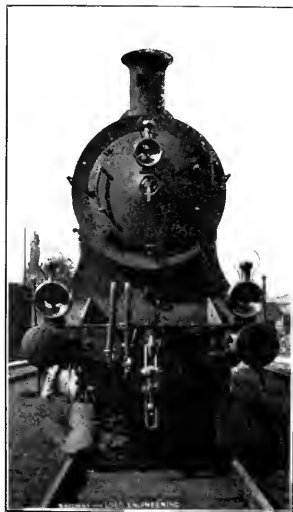
FRONT OF DURA-SIMPLON RAILROAD EXPRESS ENGINE WITH SNOW SCRAPPERS.
