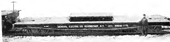
SPECIAL STEEL FLAT CAR, 120,000 LBS. CAPACITY.
