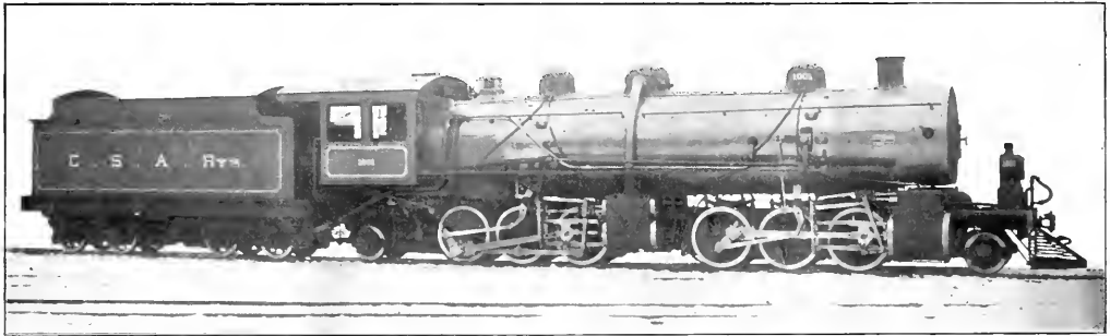
MALLET ARTICULATED COMPOUND FOR THE CENTRAL SOUTH AFRICAN RAILWAYS.
