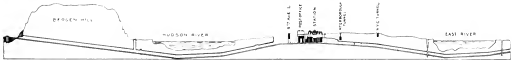
DIAGRAM OF P. R. R. TUNNEL SYSTEM FROM BERGEN HILL TO LONG ISLAND.
