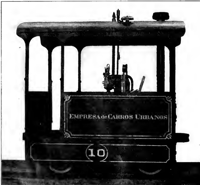
H. K. PORTER CO. STEAM MOTOR FOR STREET RAILWAY SERVICE.
