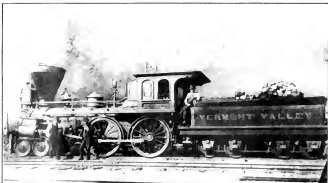
VERMONT VALLEY ENGINE WITH WHISTLE DIRECT FROM BOILER
