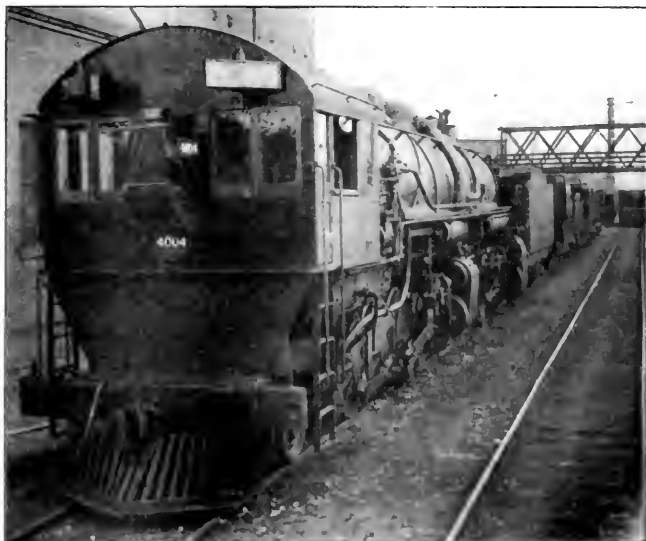
VIEW OF BALDWIN MALLET COMPOUND FOR THE SOUTHERN PACIFIC CO. THIS ENGINE RUNS CAB FIRST.
