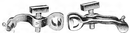
FIG. 2. LOCKING APPARATUS, GOLD STEAM COUPLING.
