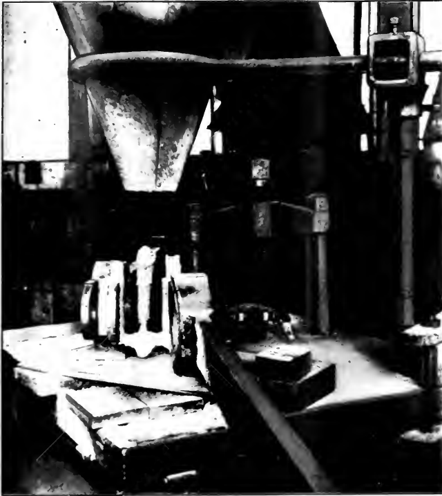
WELDING JAWS ON CLEVIS END OF SIDEROOD.
