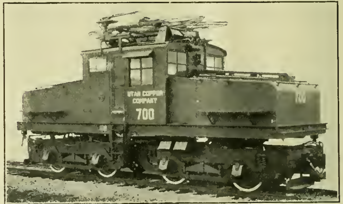
Utah Copper Company Electric Mine Locomotive Built by the General Electric Company
