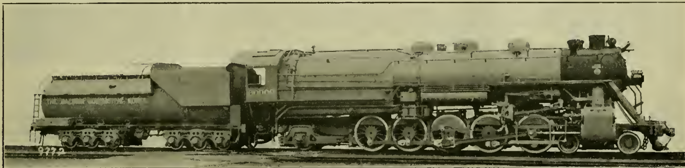
Three-Cylinder Experimental Compound Locomotive Built by the Baldwin Locomotive Works
