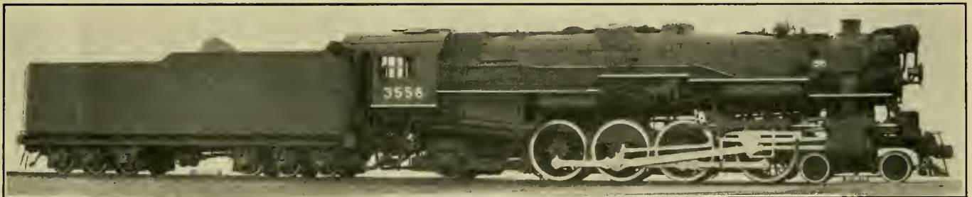
4-8-2 Type Three-Cylinder Locomotive Built by the American Locomotive Company for the New York, New Haven & Hartford Railroad
