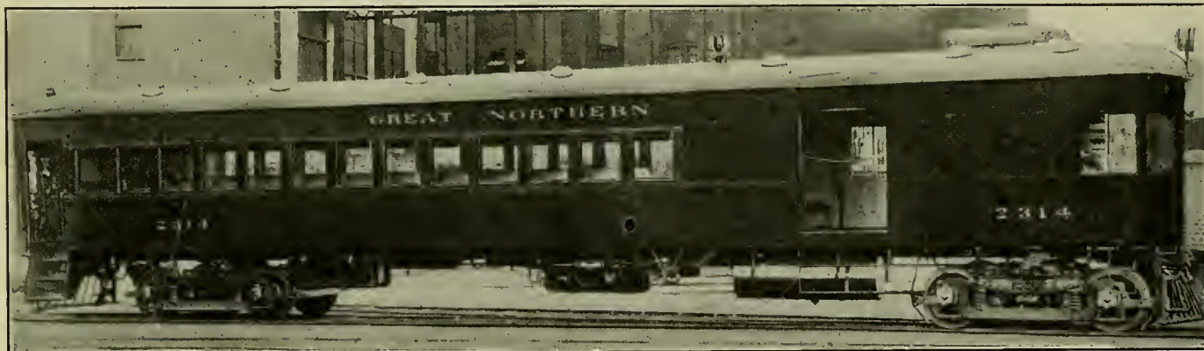
One of the Twenty-five Gas-Electric Cars in Service on the Great Northern Railway
