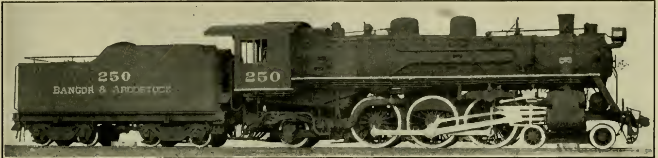
4-6-2 Type Locomotive of the Bangor & Aroostook Railroad, Built by the American Locomotive Company
