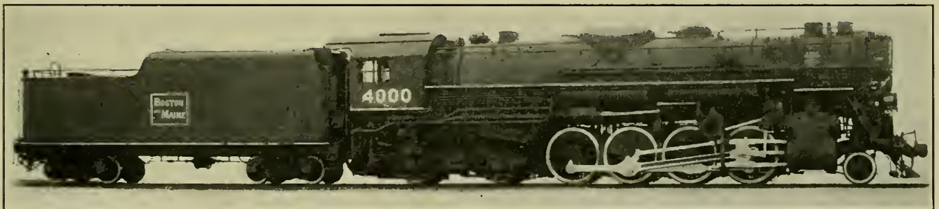
New 2-8-4 Type Locomotive of the Boston & Maine Railroad Built by the Lima Locomotive Works, Inc.
