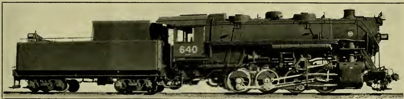
New Eight-Wheel Switch Engine of the Boston & Maine—Built by the Baldwin Locomotive Works
