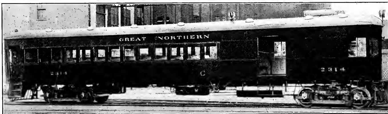
One of the Twenty-five Gas-Electric Cars in Service on the Great Northern Railway
