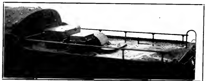
Rear of Tender Showing Radio Equipment and Antenna
