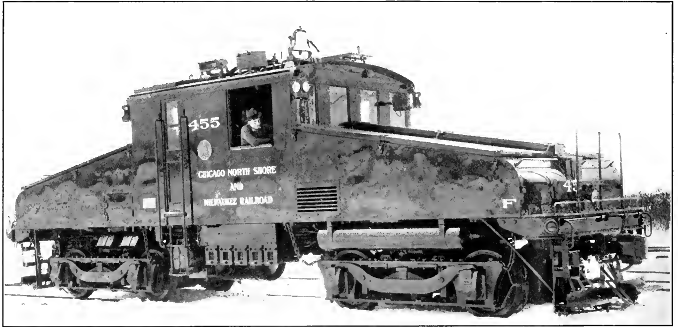
Electric Locomotive on the Chicago, North Shore and Milwaukee Railroad—Can Operate From Trolley or Storage Battery Power
