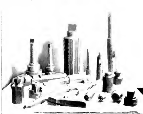
Fig. 4—Group of Tools in Which Casehardened Machine Steel Has Been Used with Success
