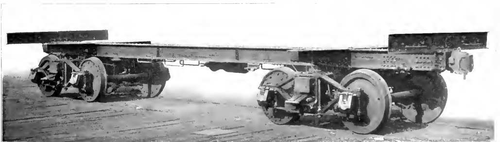
The Steel Members of the Underframe of the Erie Caboose
