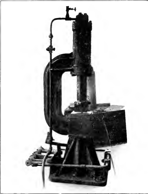
Pneumatic Hammer Used in Reclaiming Track Spikes
