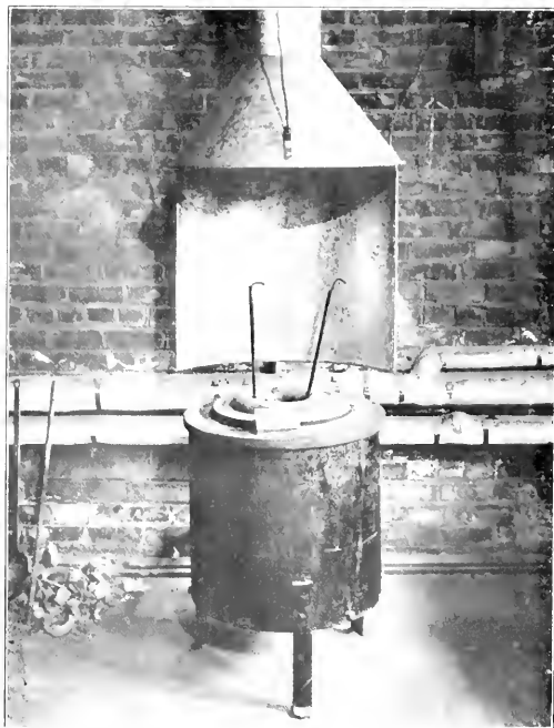
Method of Temperature Indication in Metal or Salt Bath Furnace
