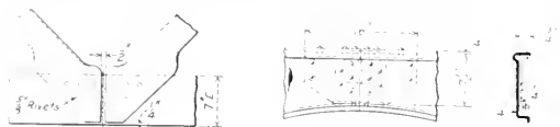
Details Showing Diagonal Brace Connection to Side Sill and Side Plate Splice
