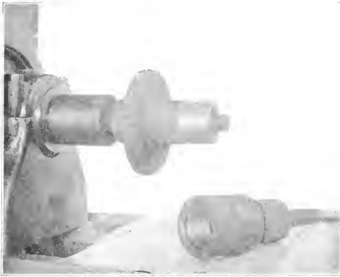
Tank Valve Casting Mounted on Expanding Mandrel for Finishing Hose Nut End
