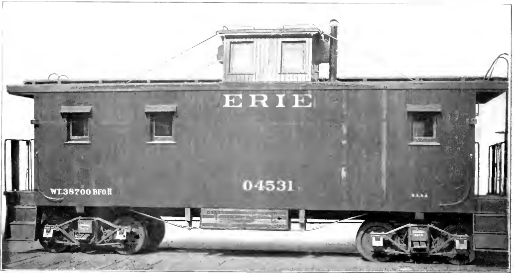
Wooden Caboose with Steel Center Sills and Body Bolsters
