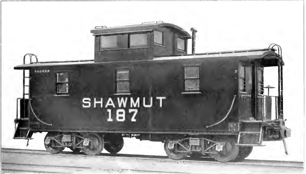
Steel Underframe Caboose in Service on the Pittsburg, Shawmut & Northern; the Springs Used Are Double Elliptic Instead of the Helical Springs Shown
