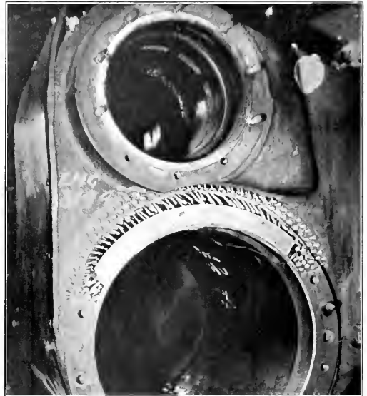
Fig. 9—Cylinder Prepared for Welding
