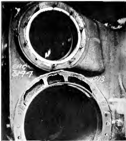
Fig. 8—Broken Cylinder Repaired by Arc Welding
