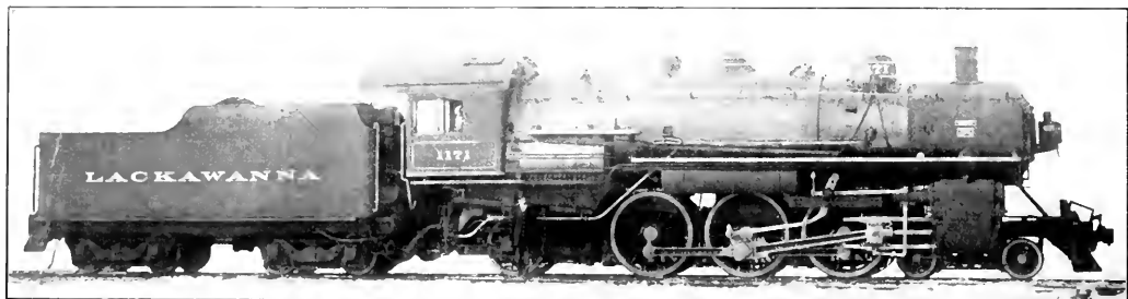
Lackawanna Pacific Type Locomotive, the Boiler of Which Has a Water Tube Firebox
