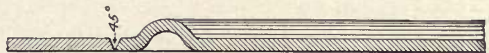
Fig. 424—Partial View of Patch About to Be Welded to the Side Sheet.
