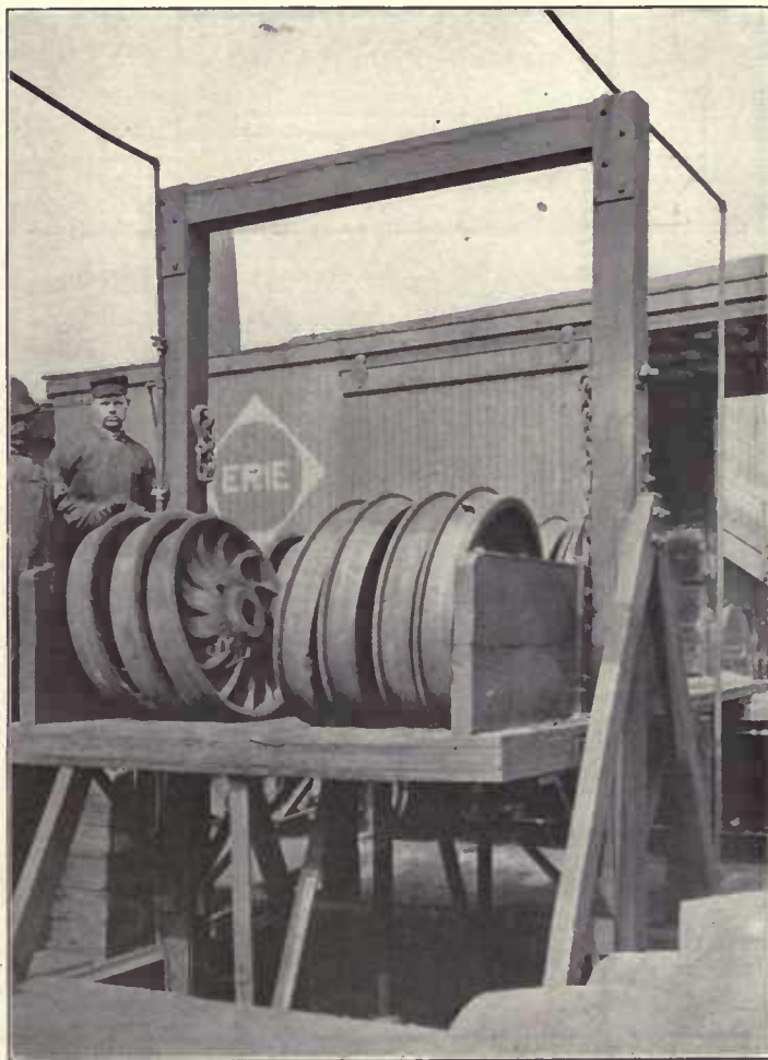
Fig. 624—Wheel Hoist Raised to Level of Car Floor.
