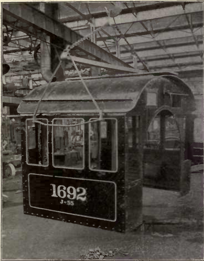
Fig. 255—Device for Handling Steel Cabs.
