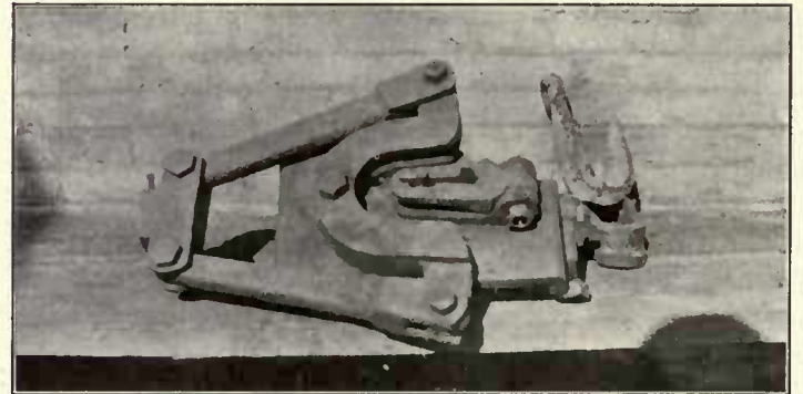
Fig. 465—Hook Bending Machine at Close of Operation.
