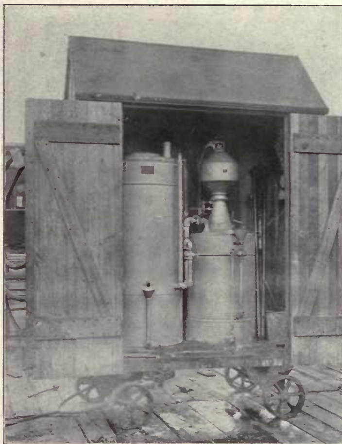
Fig. 436—Acetylene Generator Mounted on a Truck.
