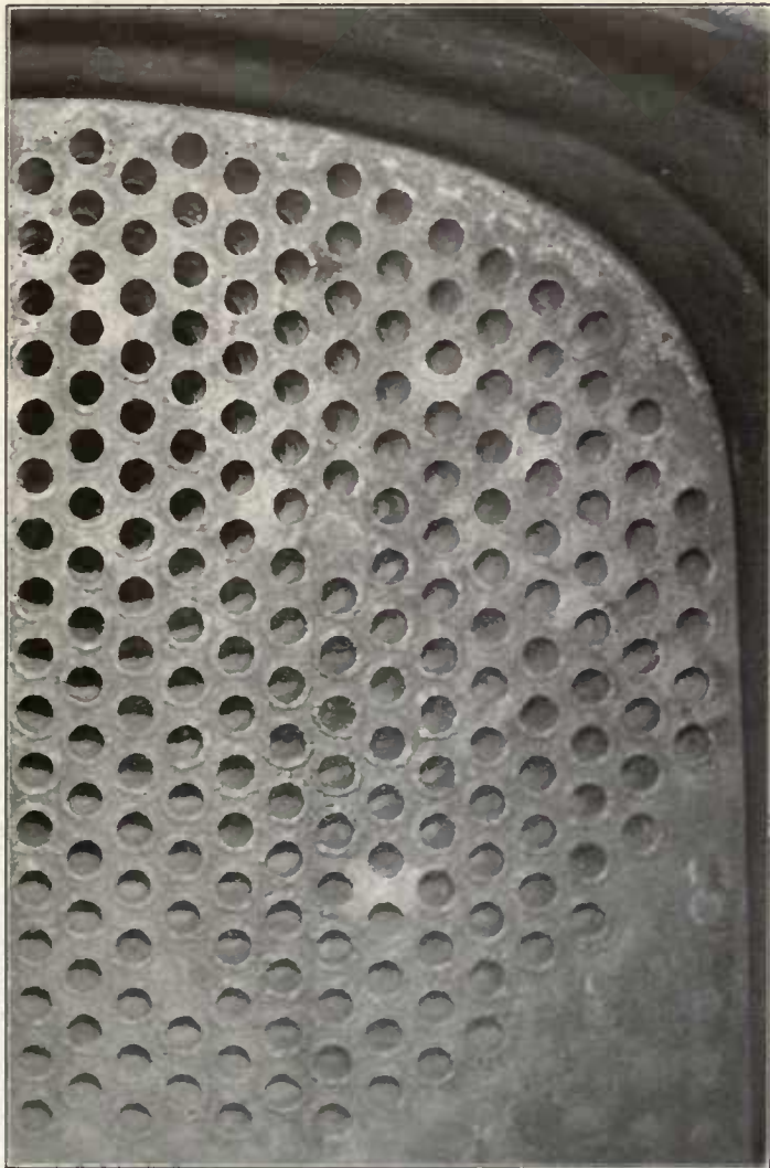
Fig. 411—Boiler Tubes Welded in Flue Sheet of Jacobs-Shupert Firebox.
