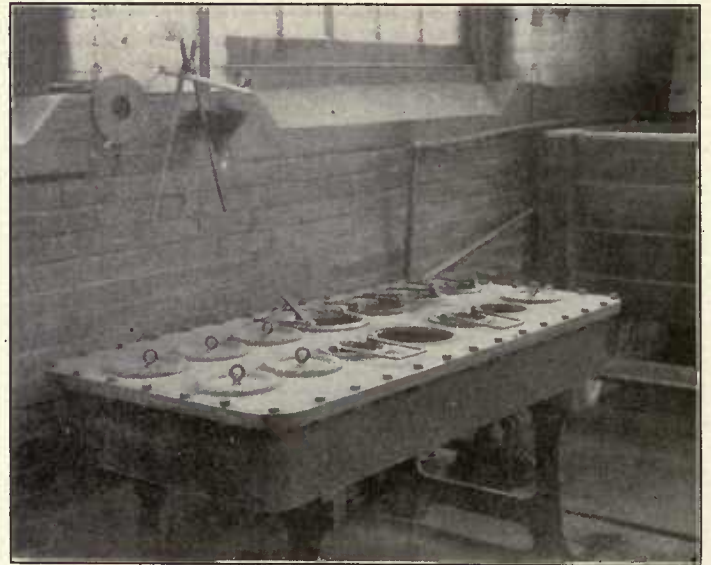
Fig. 663—Glue Pot in Cabinet Shop.
