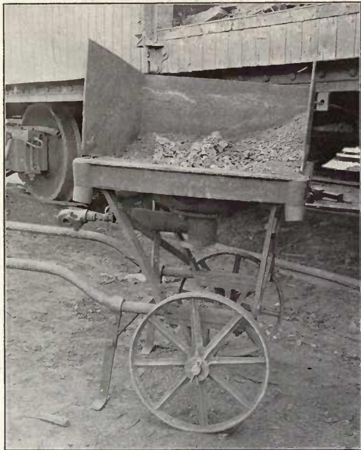
Fig. 644—Portable Rivet Heater.
