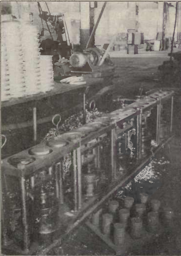
Fig. 157—Molds for Pouring and Machine for Finishing Piston and Valve Rod Packing Rings.
