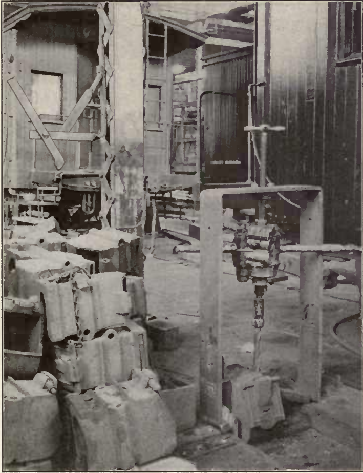
Fig. 612—Device Used for Drilling Journal Box Bolt Holes; also Metal Scaffold Bracket Used in Freight Car Shop.
