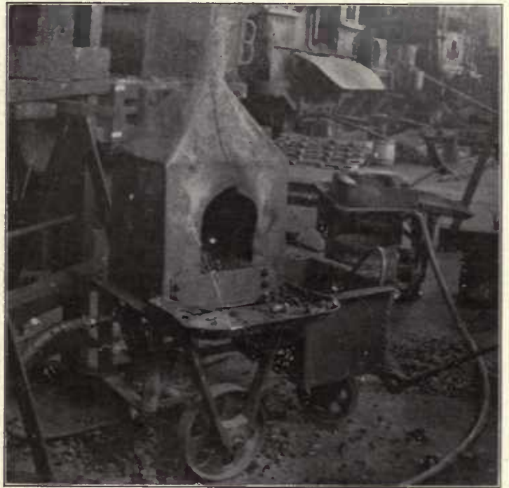
Fig. 348—Portable Rivet Forge.
