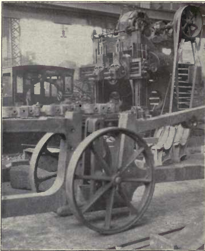
Fig. 458—Truck for Transporting Locomotive Frames.
