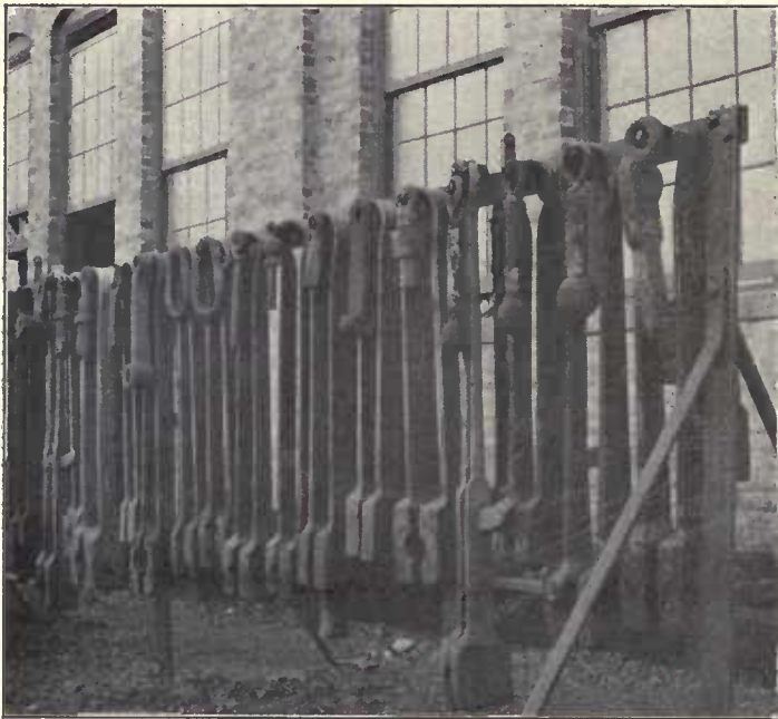
Fig. 482—Rack for the Storage of Steam Hammer Formers.
