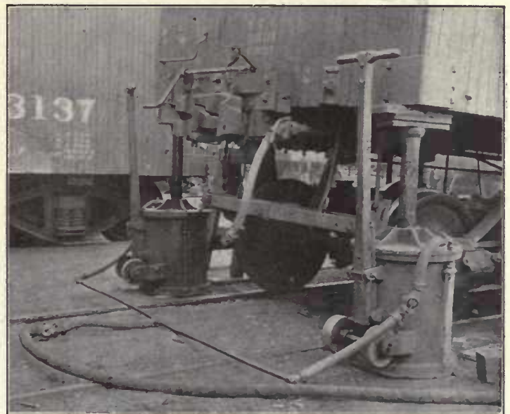
Fig. 607—Air Jacks for Loaded Cars.
