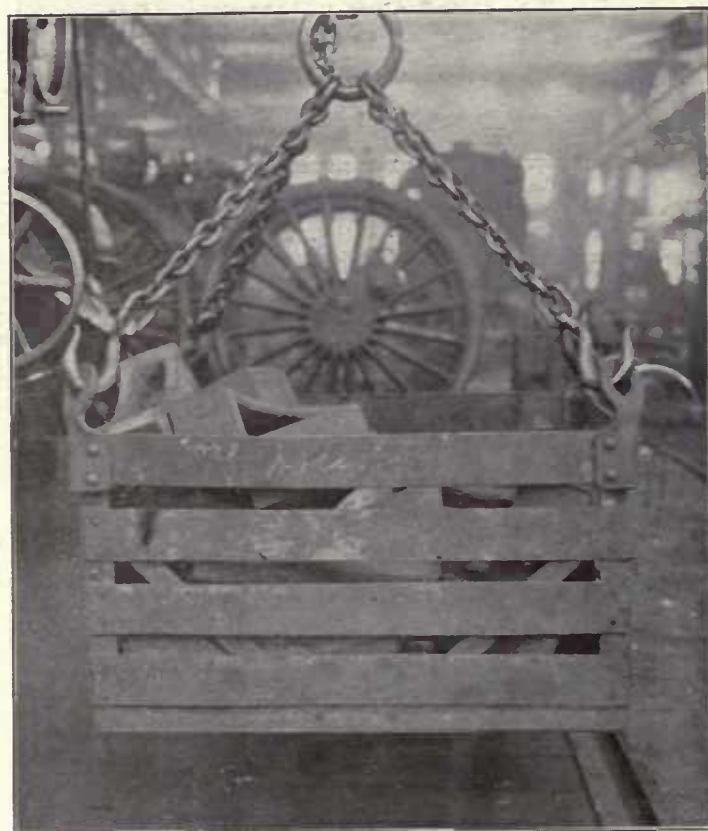
Fig. 788—Metal Crate for Handling Material.
