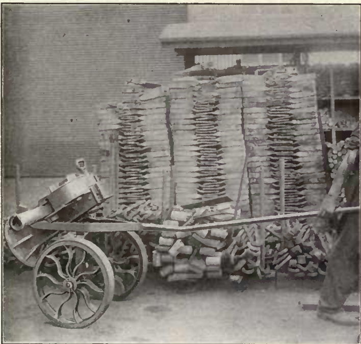
Fig. 605—The Jack in Position on the Buggy.
