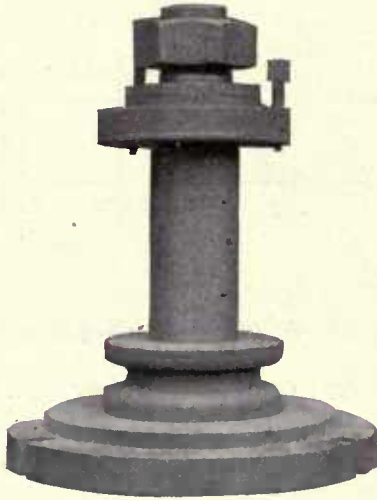
Fig. 60—Chuck for Turning Driving Box Brasses.
