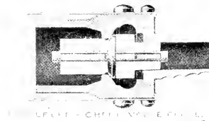
First Form of Hose Coupling with Check Valves "Straight Air" Brake of 1869.
