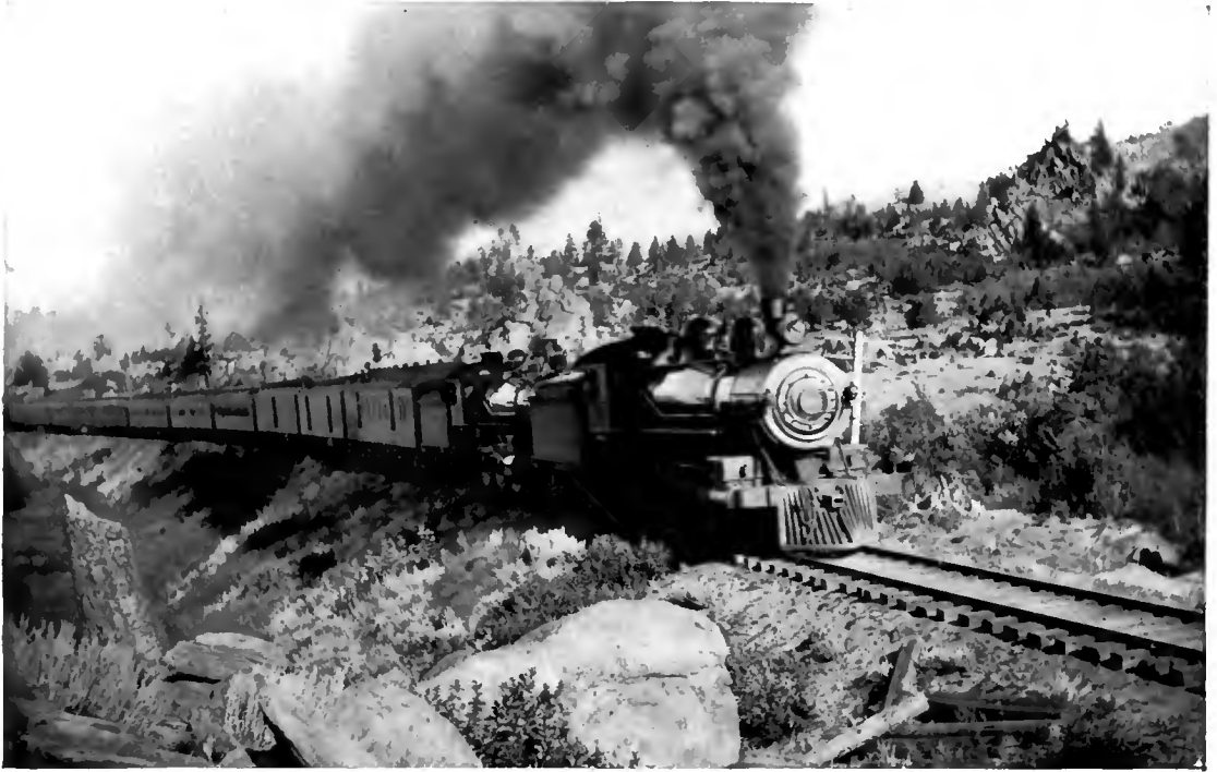
THE NORTHERN PACIFIC TRANSCONTINENTAL EXPRESS CLIMBING THE 116 FEET PER MILE GRADE THROUGH THE ROCKIES WITH A "DOUBLE-HEADER."
