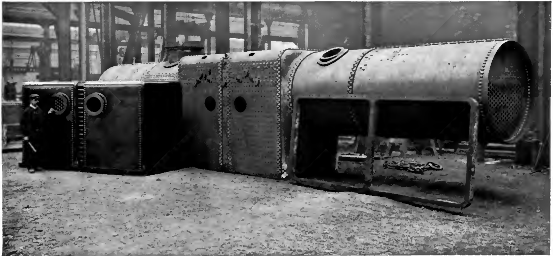
THE DOUBLE BOILER, FIRE-BOXES, AND FOUNDATION RING OF THE LARGE "FAIRLIE" ENGINE BUILT FOR THE MEXICAN RAILWAY.
