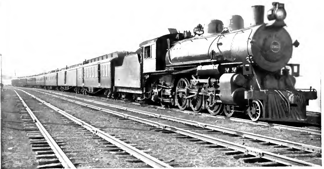
THE NORTH COAST "LIMITED" LEAVING ST. PAUL. Drawn by the latest type of Pacific (4-6-2) engine.
