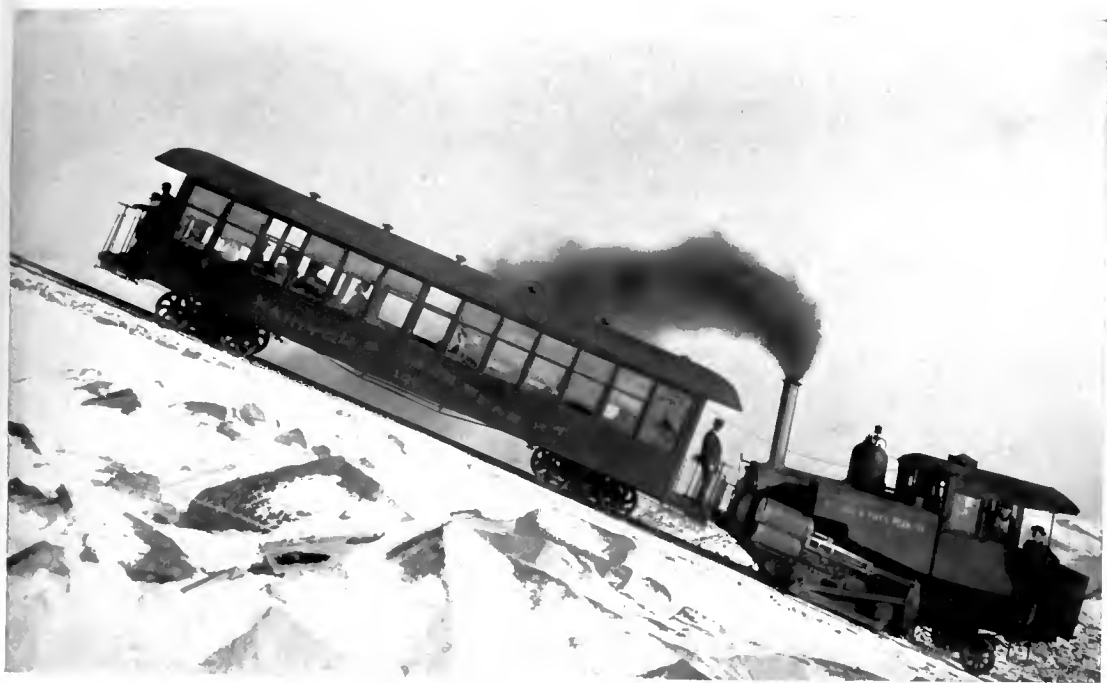
ON THE STEEPEST PART OF THE RAILWAY ABOVE THE TIMBER LINE, WHERE IT RISES 1 IN 4, SHOWING THE SPECIAL TYPE OF LOCOMOTIVE.
