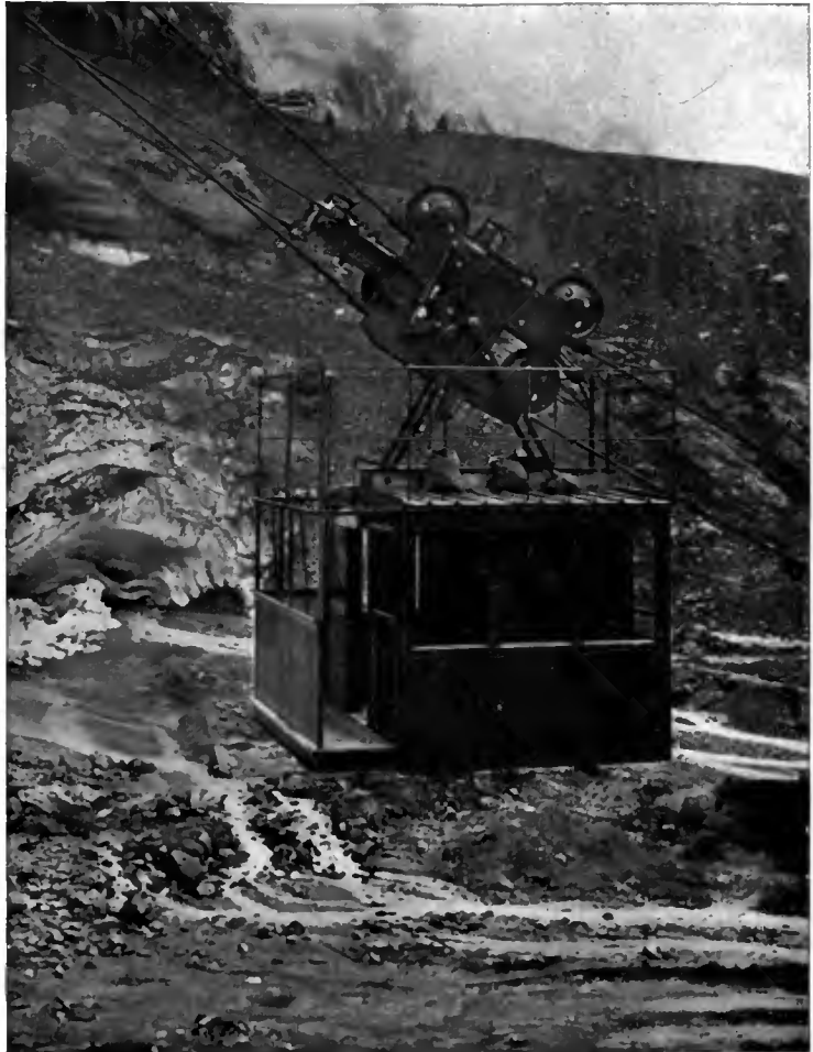
A CAR ON THE WETTERHORN AERIAL RAILWAY. The two cables forming the track are mounted one above the other.
