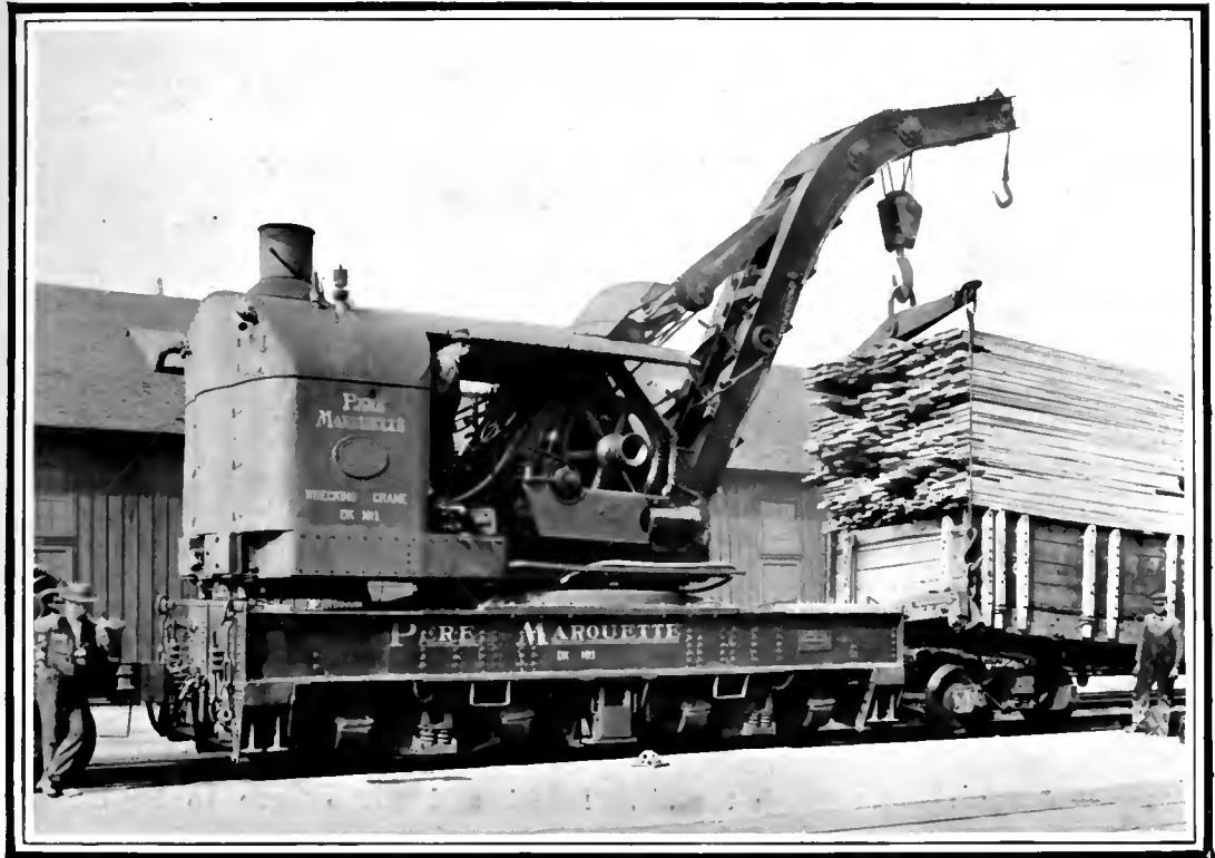
AN INDUSTRIAL WORKS' BREAKDOWN CRANE LIFTING A WAGON BODY AND ITS LOAD TO AFFORD ACCESS TO THE WHEEL TRUCK.
