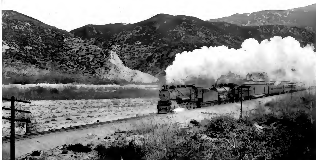
THE ATCHISON, TOPEKA, AND SANTA FÉ "CALIFORNIA LIMITED" MAKING SPEED OVER THE HEAVY GRADE OF 158.4 FEET PER MILE THROUGH THE CAJON PASS.
