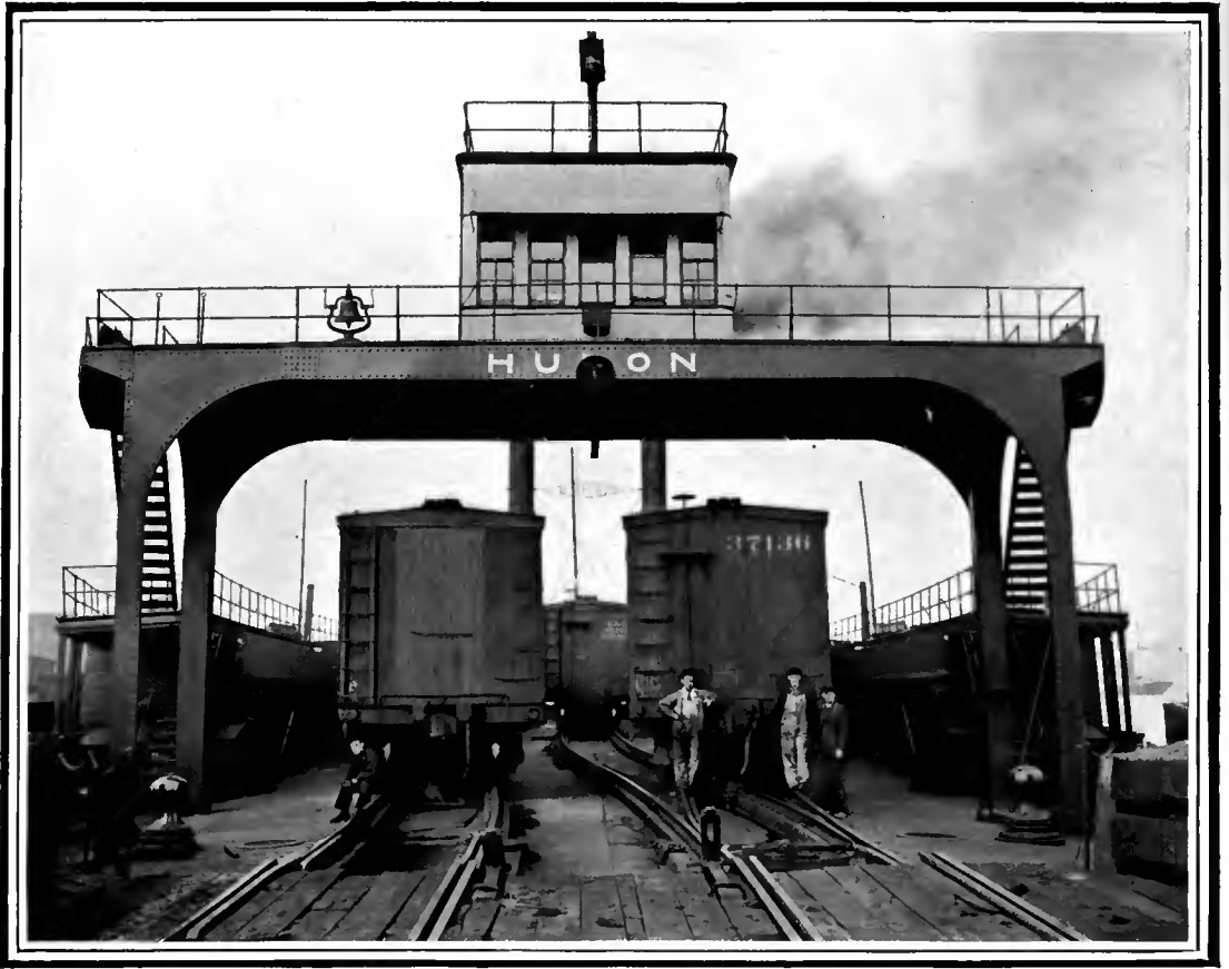
THE TRAIN DECK OF THE HURON , WHICH PLIES ACROSS THE DETROIT RIVER BETWEEN WINDSOR AND DETROIT.
