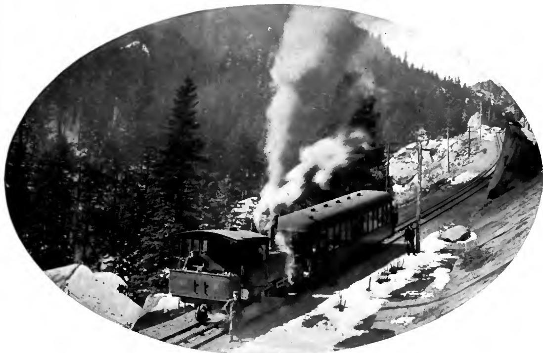
VIEW OF THE TRACK OF THE PIKE'S PEAK RAILWAY, SHOWING THE RACK-RAIL.
