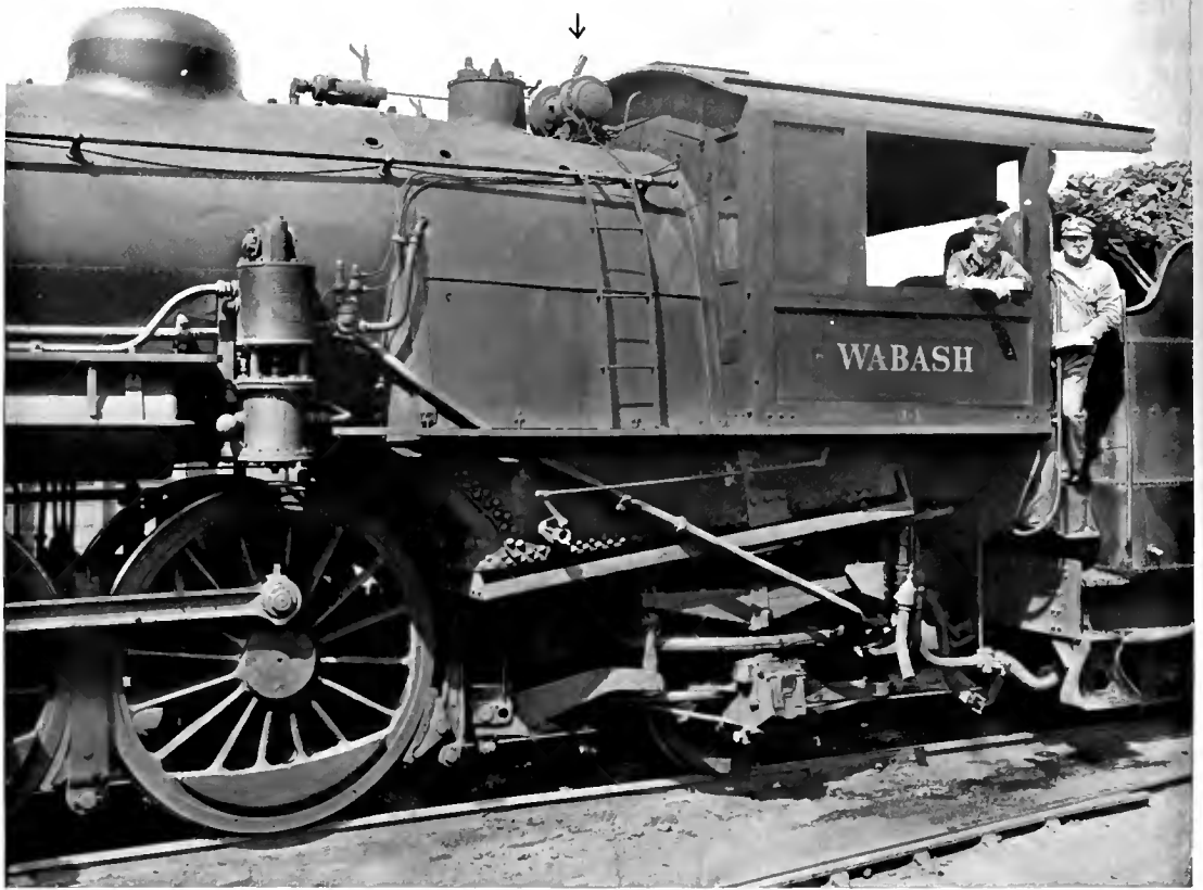
A LOCOMOTIVE FITTED WITH DYNAMO (MARKED BY ↓) FOR HEADLIGHT.
