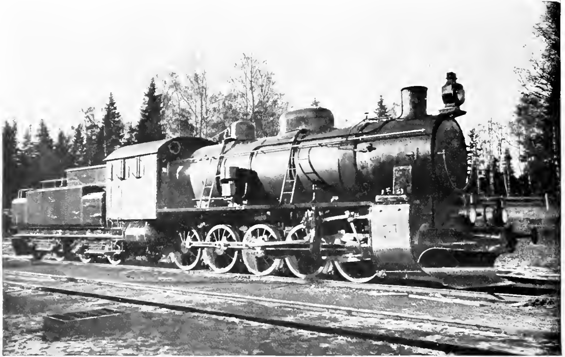
HEAVY TEN-WHEELED-COUPLED LOCOMOTIVE USED IN THE IRON ORE TRAFFIC OF SWEDEN. The engine weighs 83\frac{1}{2} tons, the whole of which is available for adhesion.
