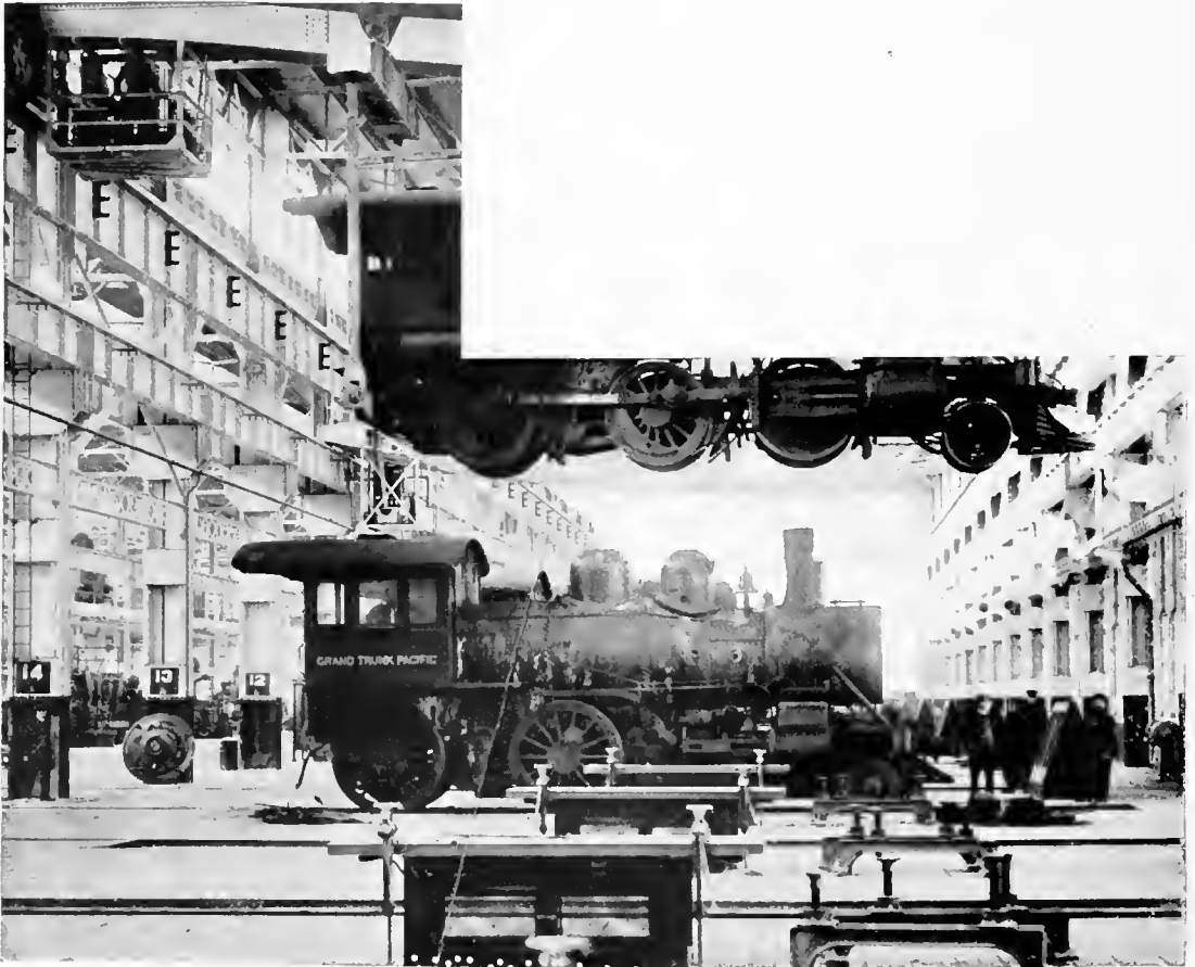
SLINGING A 100-TON LOCOMOTIVE.
