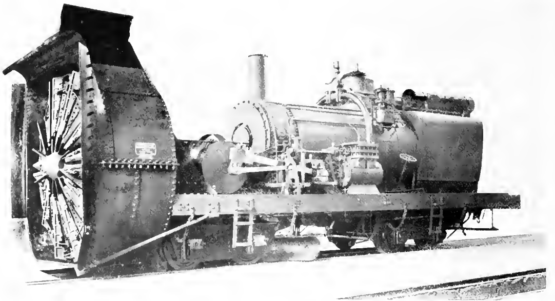
FRONT VIEW OF UNHOUSED ROTARY, SHOWING SCOOP WHEEL AND ITS DRIVING GEAR.
