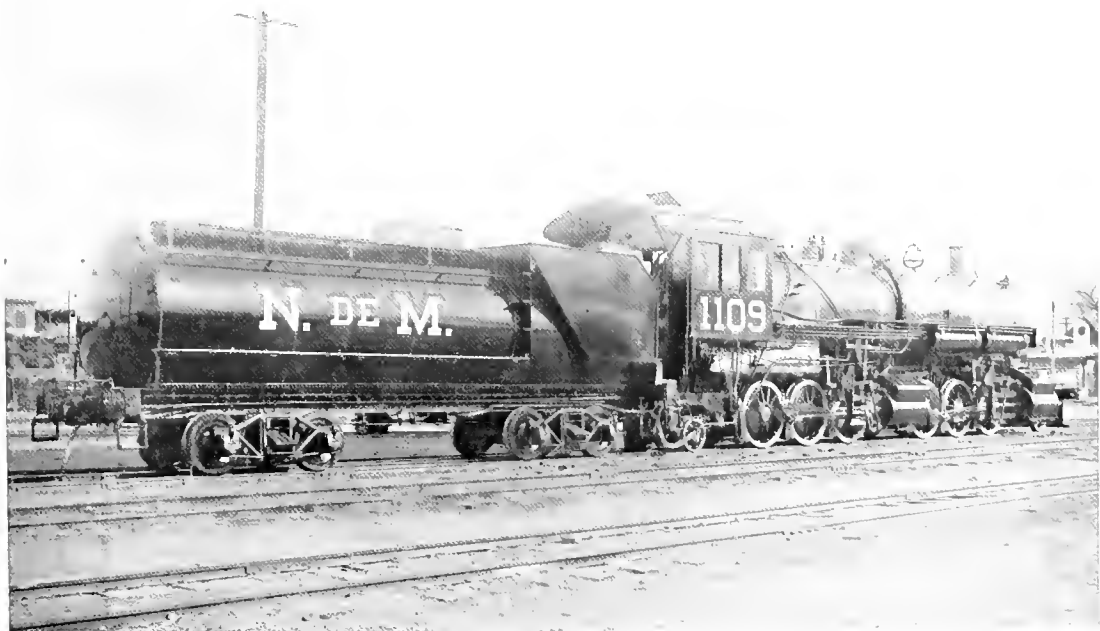
ANOTHER VIEW OF THE GIANT MALLET LOCOMOTIVE. The tender carries 7,500 gallons of water, and 3,300 gallons of oil.
