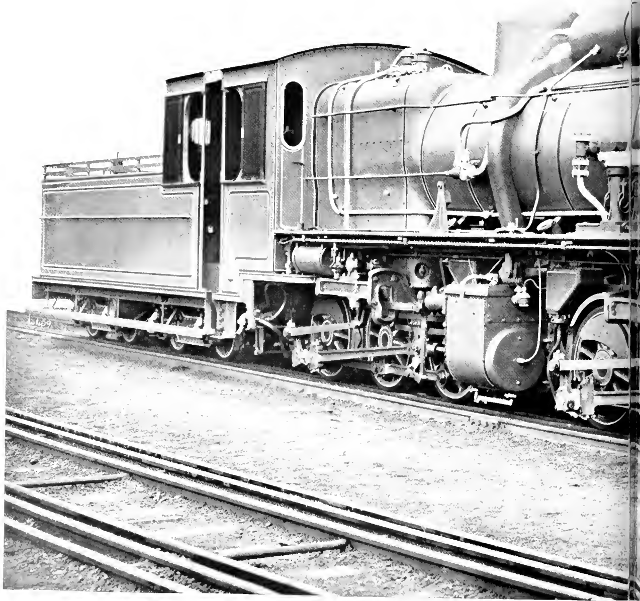
THE HEAVY 0-6-6-0 BRITISH-BUILT COMPOUND The complete narrow gauge locomotive, ready for the road, weighs 91 tons 11 cwt.
