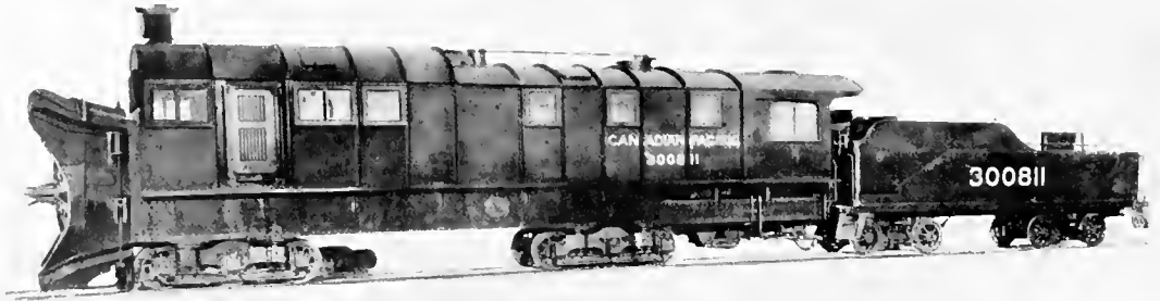
SIDE VIEW OF THE HUGE ROTARY SNOW-PLOUGH BUILT BY THE CANADIAN PACIFIC RAILWAY FOR SERVICE AMONG THE ROCKY MOUNTAINS
