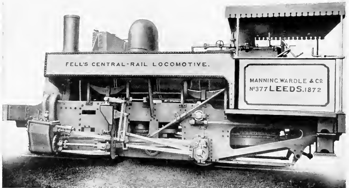
AN EARLY TYPE OF THE FELL CENTRE-RAIL LOCOMOTIVE.
