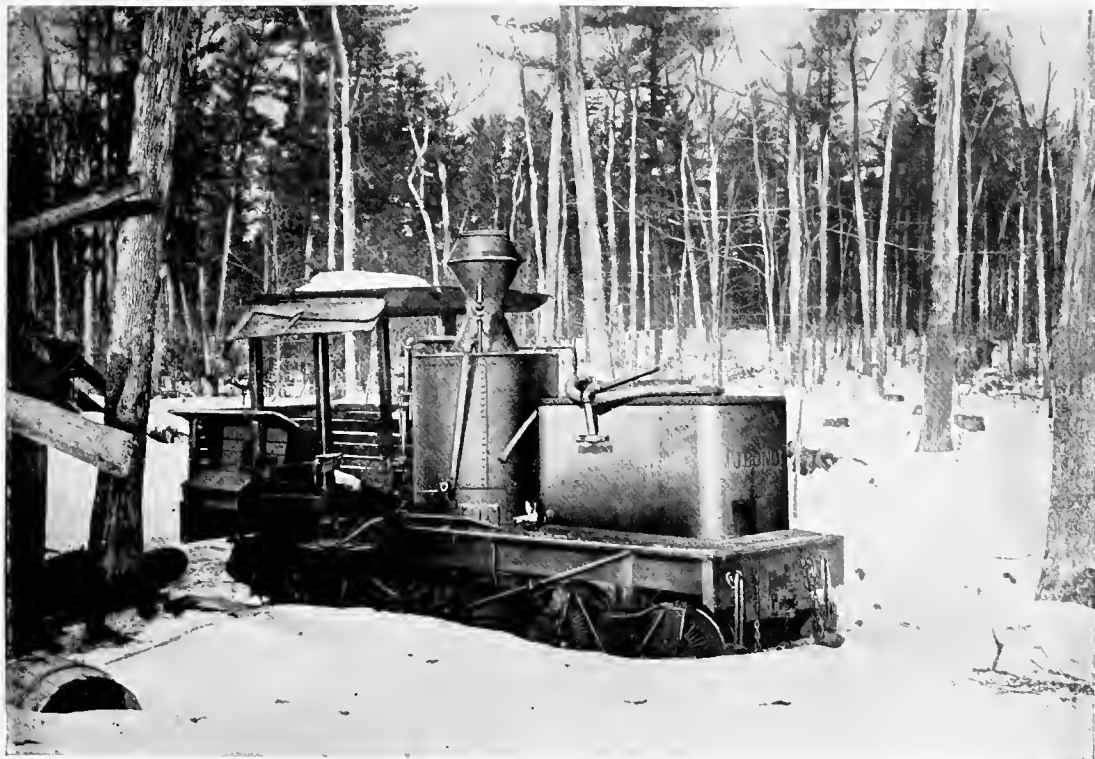
THE "M. J. BOND," ONE OF THE EARLIEST GEARED LOCOMOTIVES BUILT BY MR. EPHRAIM SHAY FOR LOGGING IN MICHIGAN
