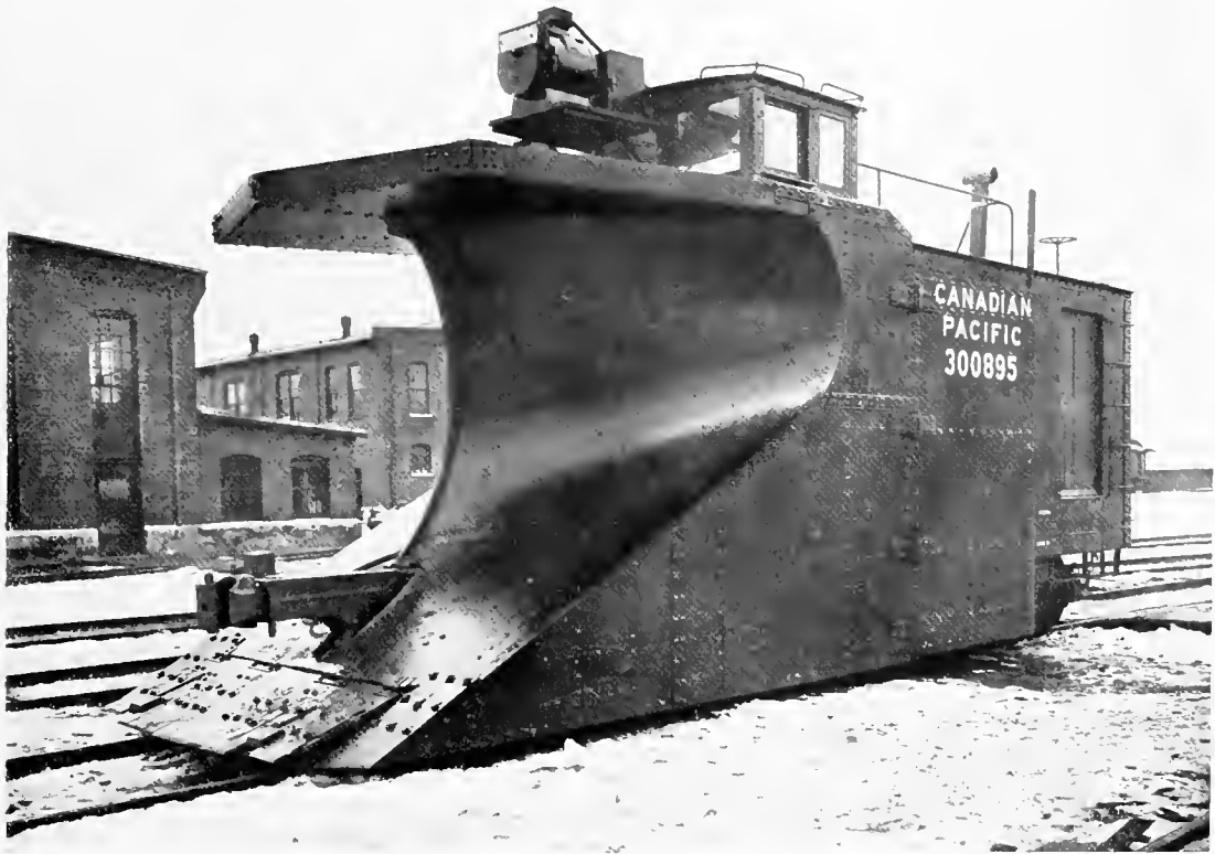
FRONT END OF WEDGE SNOW-PLOUGH USED UPON THE CANADIAN PACIFIC RAILWAY.
