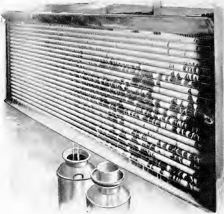
VIEW OF MILK AERATOR IN OPERATION.
