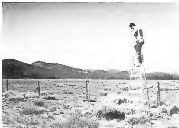
FIGURE 2.—Near-vertical ground photographs of marked targets are taken on or near the day of the photo mission, and make up a vital part of the ground truth. Note low-flying photo plane.
