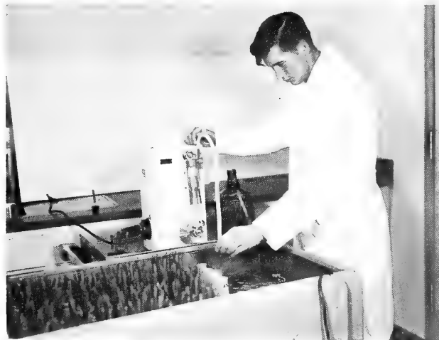
FIGURE 3.—Water bath used for incubation during an in vitro fermentation trial.
