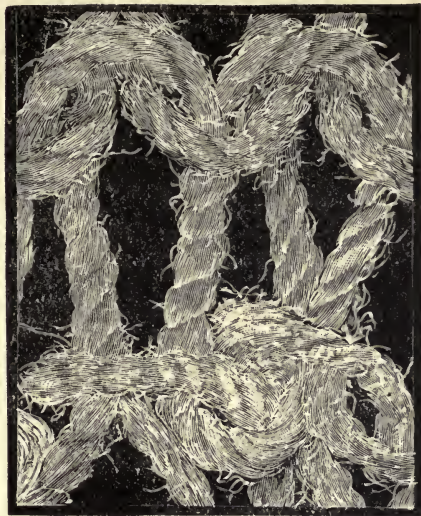
FIG. 7.—Cotton after Burning Off.
