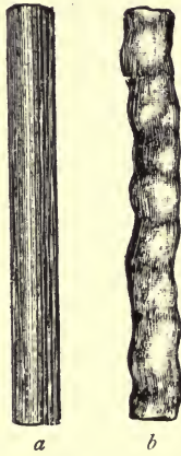
FIG. 32.—Tantalum Filament (a) before and (b) after Use on Direct Current Circuit.
