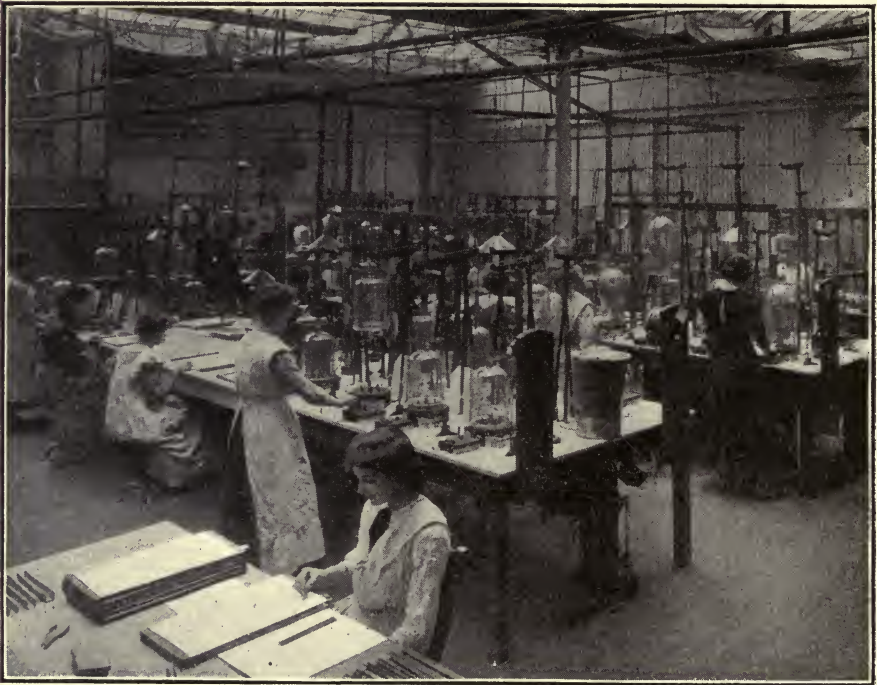
FIG. 27.—"Flashing" Room at Messrs Edison & Swan's Works.
