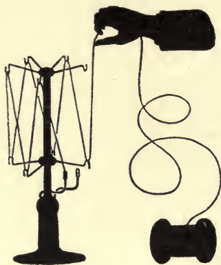
FIG. 29.—Method of Arranging Continuous Filament on "Spider."
