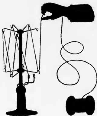
FIG. 29.—Method of Arranging Continuous Filament on "Spider."
