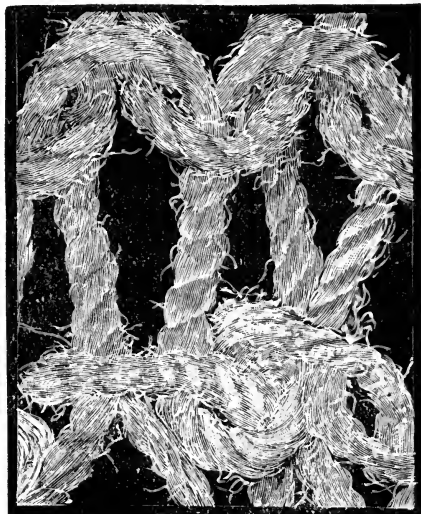
FIG. 7.—Cotton after Burning Off.
