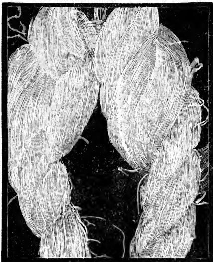
FIG. 6.—Cotton before Burning Off.
