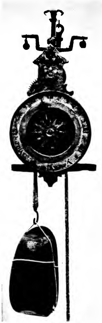
GOTHIC CLOCK, dating from the early 16th century, was photographed at the Smithsonian Institution. Stone at bottom is the driving weight; arm at top is part of escapement. Clockworks were among earliest examples of well-ordered machines.
