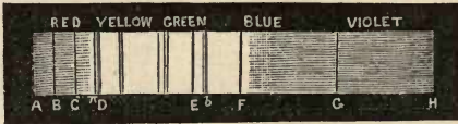
FIG. 8.—Diagram of the solar spectrum, showing the order of colour and the position of the principal absorption lines.
