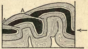
FIG. 46.—Production of thrust-planes. The strata represented are layers of clay and sand separated by cloth; they were laid down horizontally, and ridged into the position shown by a thrust acting in the direction of the arrow.
