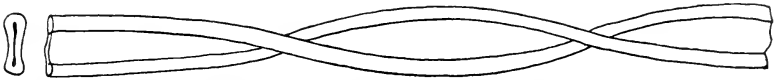
FIG. 82.—Normal cotton hair, showing convolutions and thickened edge. (From Denham, Shirley Inst. Mem. )
