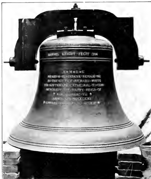
The New Tenor (50 cwt) now being erected at Southwark Cathedral.
