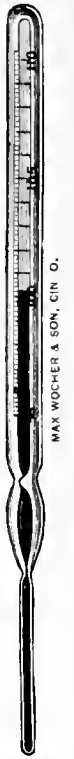
FIG. 4700.—The Minute Thermometer. The column of mercury appears magnified by means of the so-called lens front.
