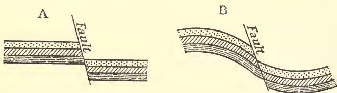
FIG. 10.—Diagrams to illustrate faults in horizontal and folded strata.
