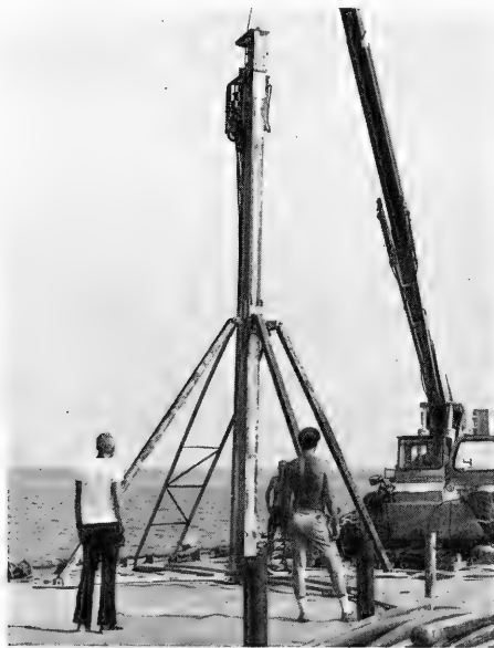
Figure 9. A 6-meter-long vibratory coring apparatus used to collect sediment cores is shown being lifted off the platform for deployment on the lake floor.
