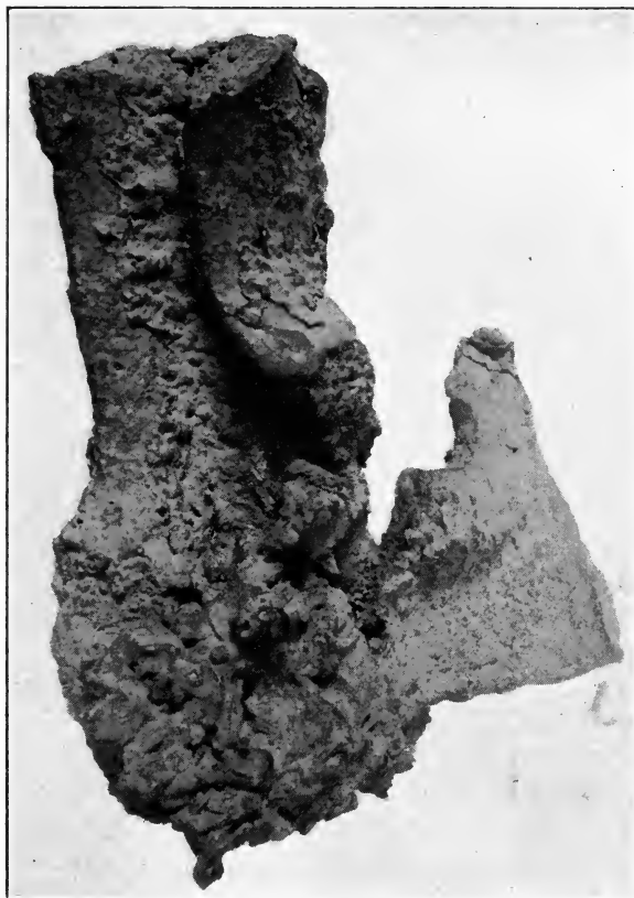
FIGURE 146. FUSED CAST-IRON PULLEY FROM THE BAYONNE FIRE.
