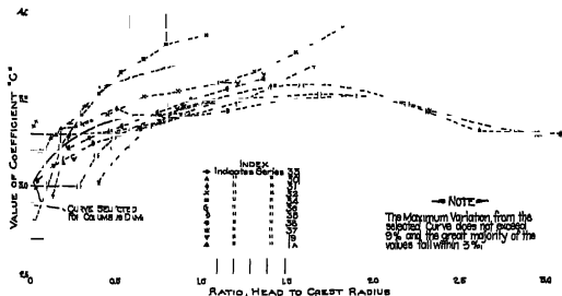
FIG. 15.—Diagram showing relation of "C" values to the ratio of head to crest radius. Experiments on curve crested dams
