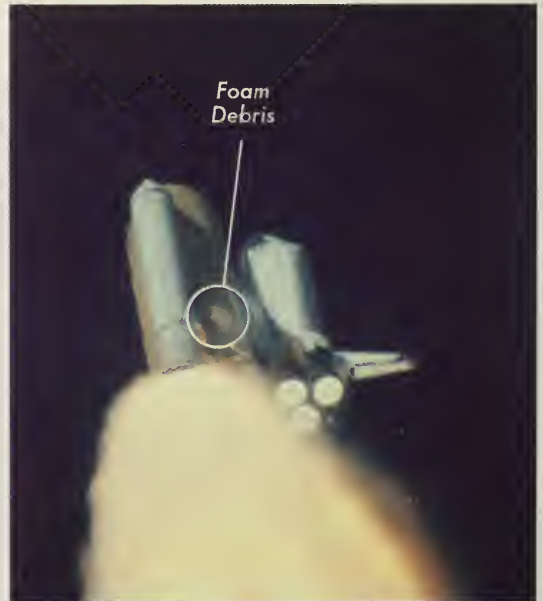
Figure 2.3-2. A shower of foam debris after the impact on Columbia's left wing. The event was not observed in real time.
