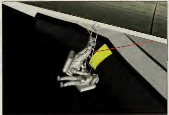
Figure 6.4-1. The speculative repair option would have sent astronauts hanging over the payload bay door to reach the left wing RCC panels using a ladder scavenged from the crew module.
