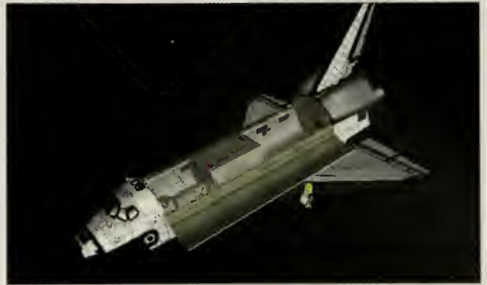
Figure 6.4-1. The speculative repair option would have sent astronauts hanging over the payload bay door to reach the left wing RCC panels using a ladder scavenged from the crew module.
