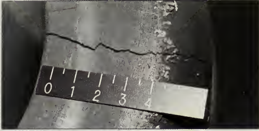
Figure 3.8-6. A 5.5-inch crack on the outboard portion of RCC Panel 6 during testing.
