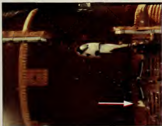
Figure 6.1-2. The first known instance of bipod ramp shedding occurred on STS-7 which was launched on June 18, 1983.
