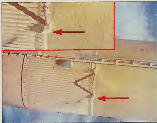
Figure 6.1-3. Only three months before the final launch of Columbia, the bipod ramp foam had come off during STS-112.
