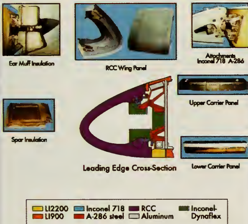
The Wing Leading Edge Structural System on Columbia.
