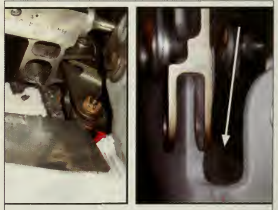
Figure 3.7-2. Each RCC panel has a U-shaped slot (see arrow) in the back of the panel. Once superheated air entered the breach in RCC panel 8, some of that superheated air went through this slot and caused substantial damage to the Thermal Protection System tiles behind this area.
