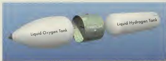
Figure 3.2-1. The major components of the External Tank.
