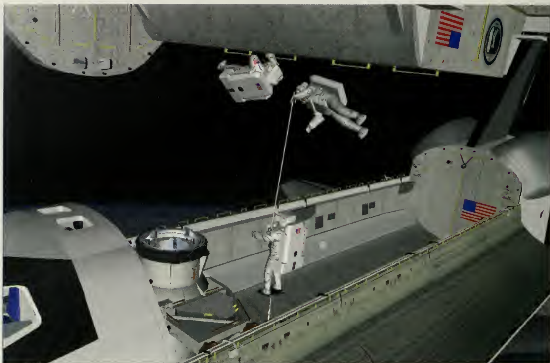
Figure 6.4-2. The rescue option had Atlantis (lower vehicle) rendezvousing with Columbia and the STS-107 crew transferring via ropes. Note that the payload bay of Atlantis is empty except for the external airlock/docking adapter.
