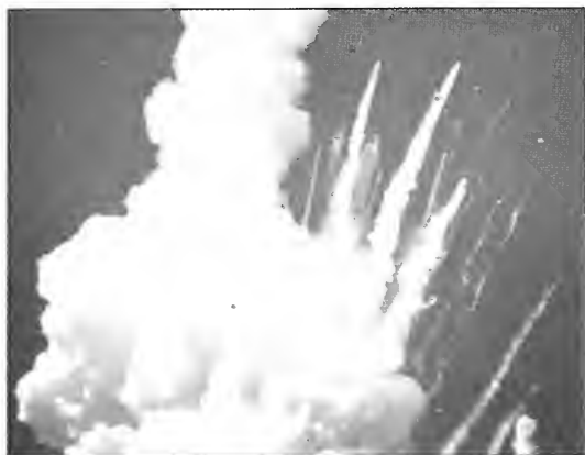
Figure 1.5-1. the Space Shuttle Challenger was lost during ascent on January 28, 1986, when an O-ring and seal in the right Solid Rocket Booster failed.
