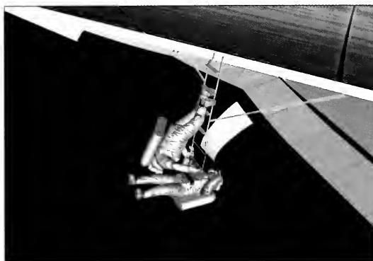
Figure 6.4-1. The speculative repair option would have sent astronauts hanging over the payload bay door to reach the left wing RCC panels using a ladder scavenged from the crew module.
