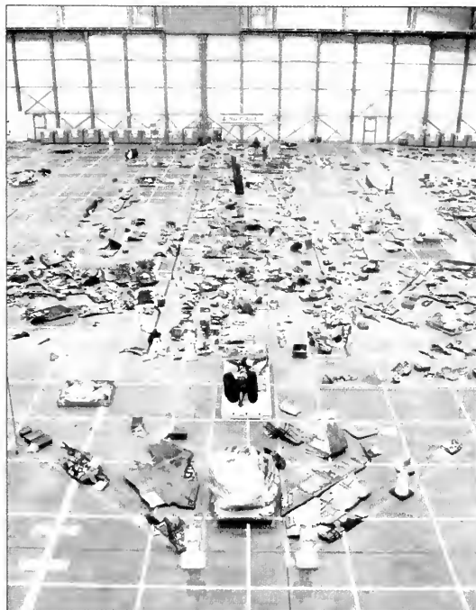
Figure 2.7-4. Recovered debris was returned to the Kennedy Space Center where it was laid out in a large hangar. The tape on the floor helped workers place each piece near where it had been on the Orbiter.
