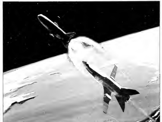
Figure 1.1-1. Early concepts for the Space Shuttle envisioned a reusable two-stage vehicle with the reliability and versatility of a commercial airliner.
