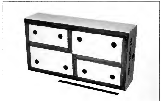
Figure 3.8-3. A typical foam projectile, which has marks for determining position and velocity as well as blackened outlines for indicating the impact footprint.
