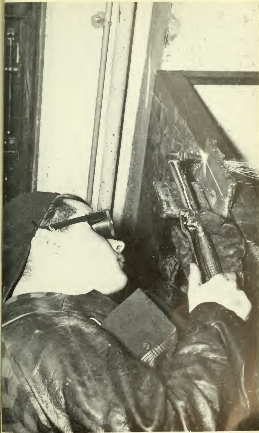
Cutting with Acetylene Torch at Welding Shop
