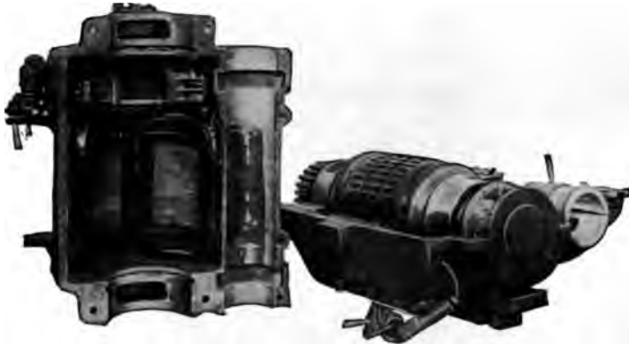
Fig. 23. — Westinghouse No. 85 Motor. (Showing Parts.)
