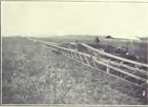
FIG. 51.—Conveyor, and cable driving eleven supporting caterpillars, also take-up mechanism for the cable.
