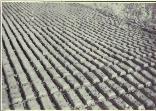
FIG. 55.—Partially air-dried peat from the new plant, showing the uniform spreading secured.
