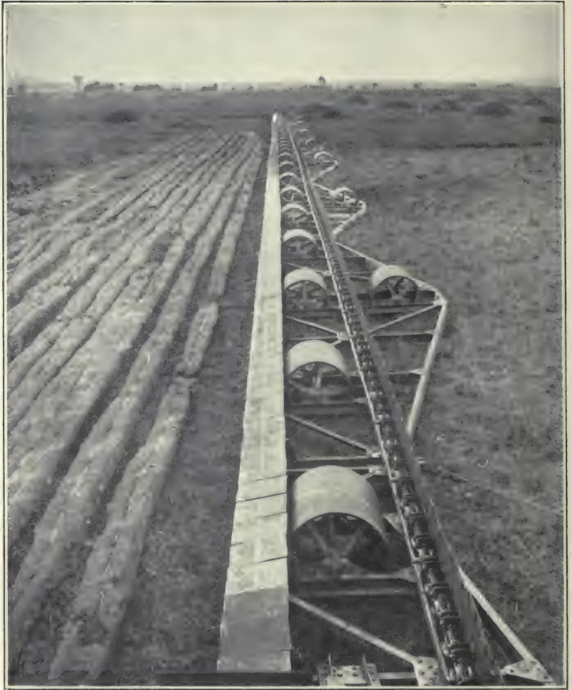
FIG. 68.—Dolberg sod transporter.
