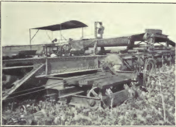
FIG. 52.—Intermediate caterpillar with driving mechanism and driving cable.
