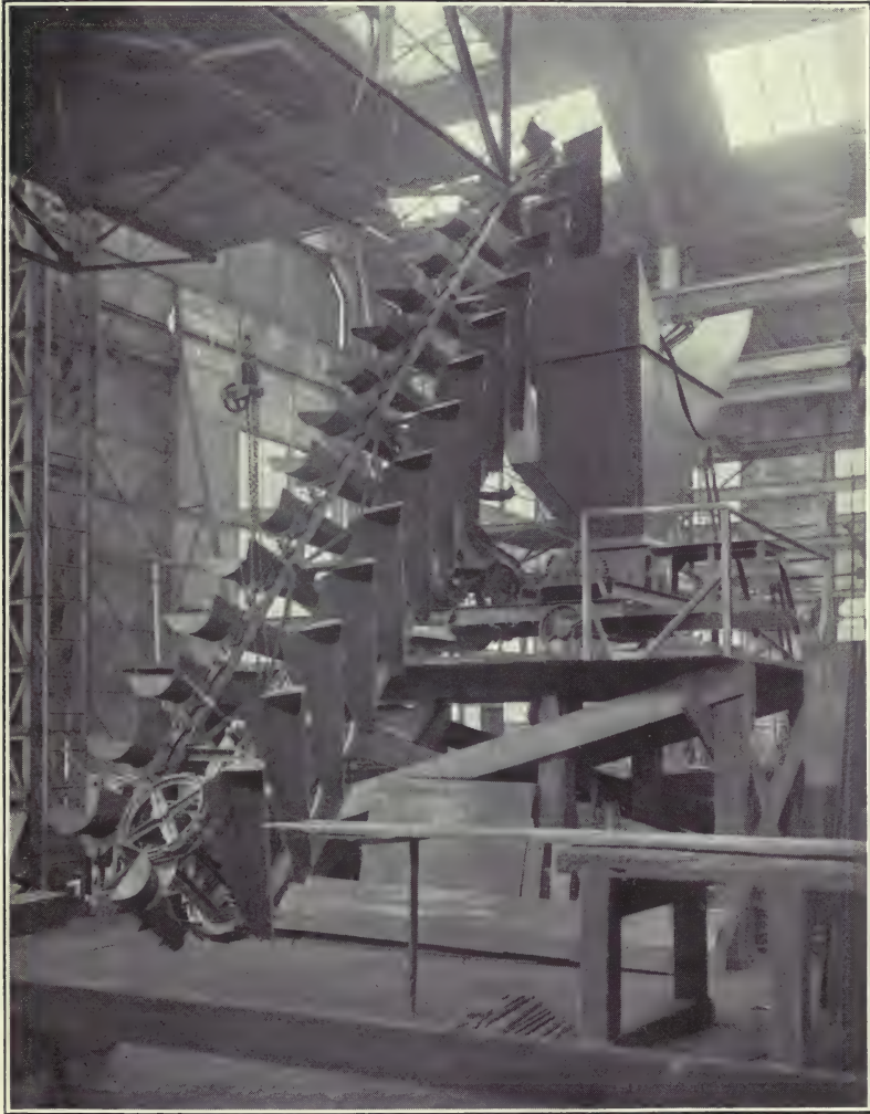
FIG. 56.—Dredger of Wielandt machine.
