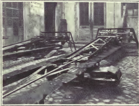
FIG. 58.—Wielandt transporter with caterpillar bearings.
