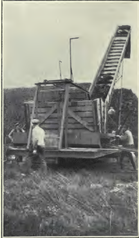
FIG. 78.—Elevator machine for stacking air-dried peat.
