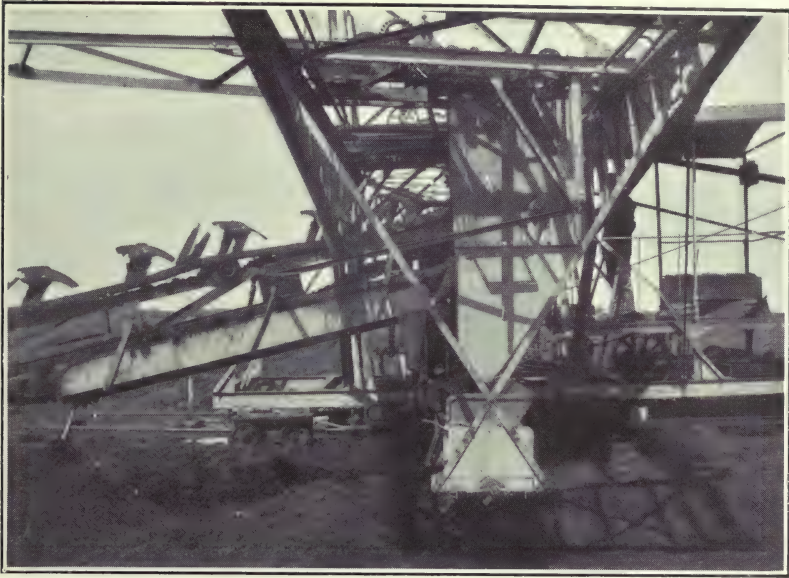
FIG. 67.—Near view of knives on excavator chain and horizontal screw conveyor.
