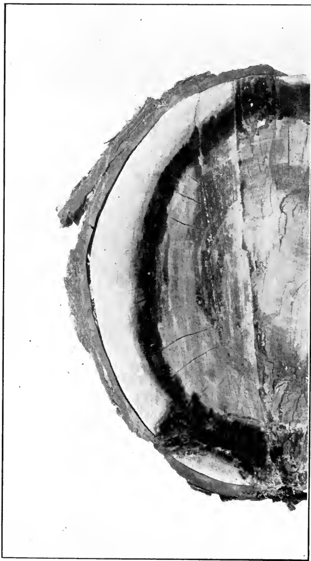
Fig. 3.—Section of Trunk of living Yellow Birch showing decay in inner sapwood and heartwood caused by the True Tinder Fungus. This section was kept for a few weeks under conditions favorable to development of fungus on the affected cut surface. The surface growth of the fungus darkened.
