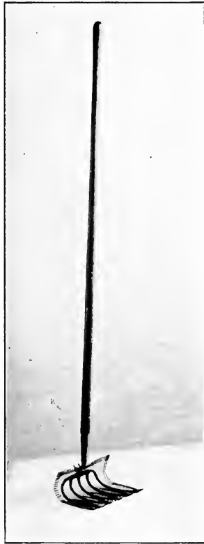
b. Potato hook with prongs covered with wire netting, for removing mud from ditches.
