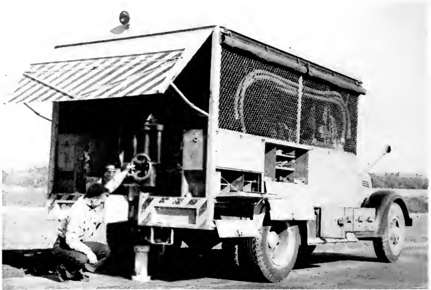
BEGINNING A CUT, THE HOLLOW CYLINDRICAL BIT IS IN CONTACT WITH THE ROAD
