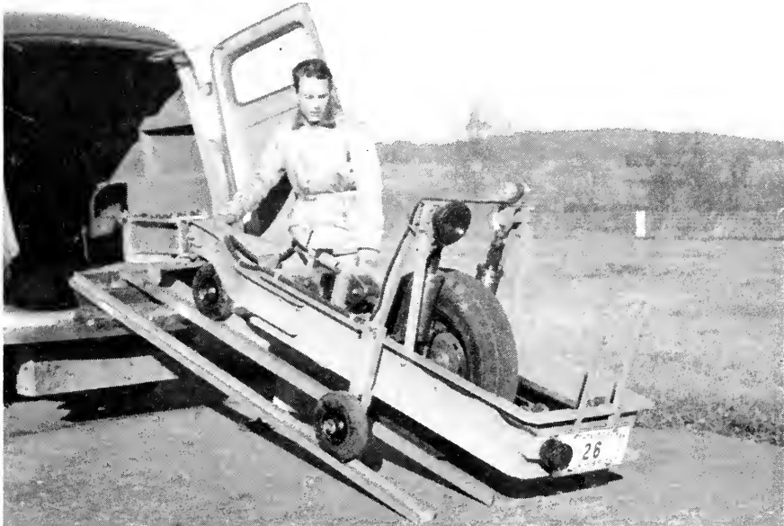
LOADED IN TRUCK. THE INDICATOR CAN BE TRANSPORTED TO ANY PART OF THE STATE—ROAD ROUGHNESS INDICATOR
