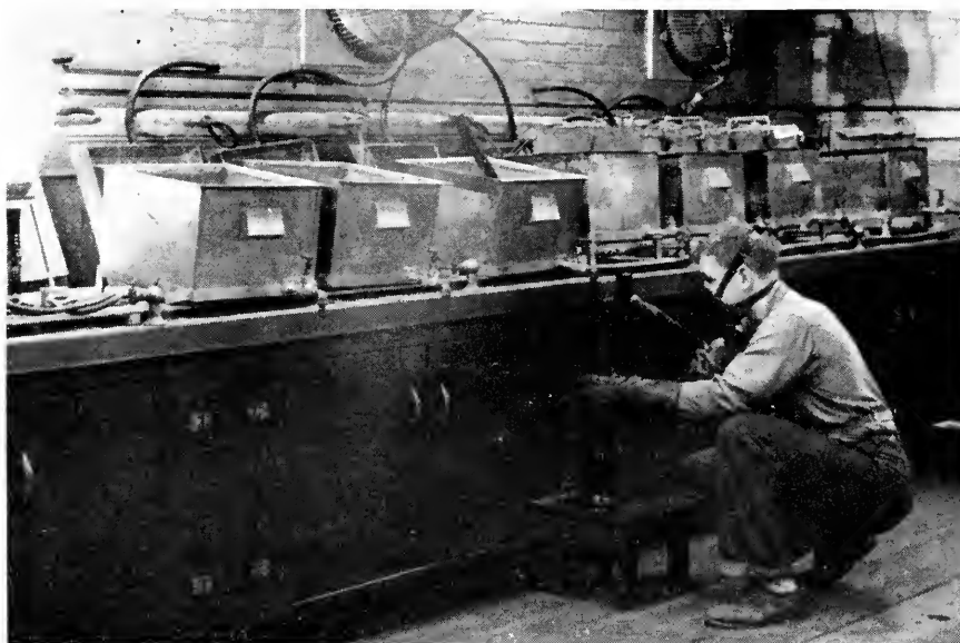
TECHNICIAN, MASKED AS PROTECTION FROM NOXIOUS FUMES, DRAWS OFF A SAMPLE OF ASPHALT LADEN SOLVENT
