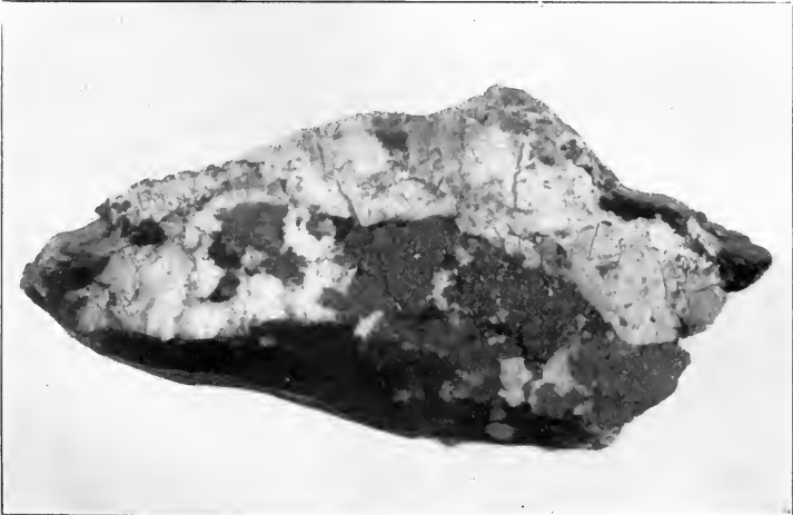
Part of a Lense of Ore, Moose River Tungsten Mines. Black Slate, Dark Grey Arsenopyrite. Clear White Quartz. The dull white forming the upper part of the picture is Scheelite.
