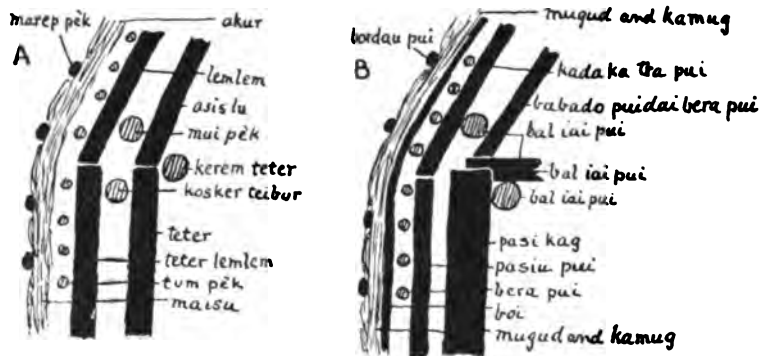
FIG. 140. Details of the construction of modern houses in Torres Straits. A, Mer; B, Mabuiag, by A. W.
