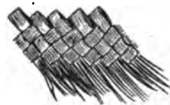
FIG. 107. Upper edge of a basket shewing method of finishing. Cf. pl. XV. fig. 1.
