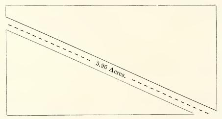
Note.—The dotted line shows the centre of the railroad track, the line of which is slightly curved.
