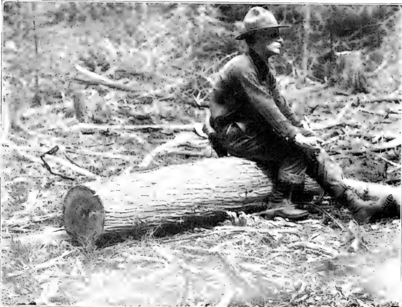
Fig. 10. Illustrating the custom of first cutting a pole to length and then butting off for defect, a practice which results in much waste. Two feet from the butt of this tree would have cleared it.
